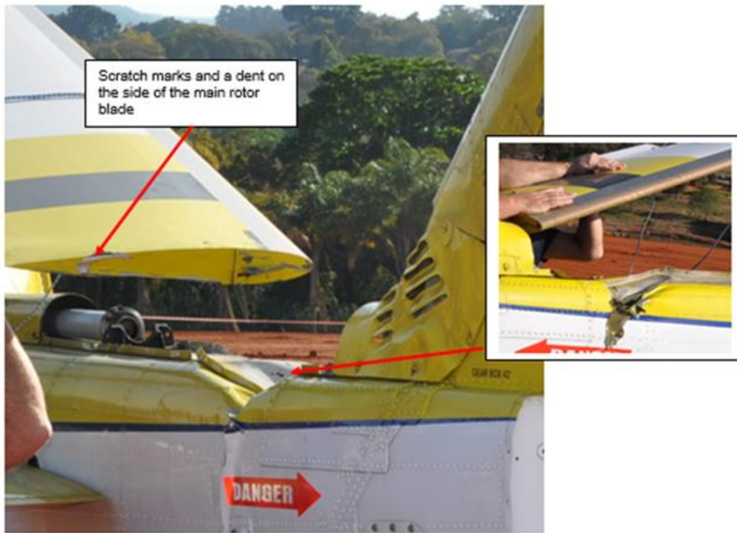
Figure 5: The severed tail drive shaft.
