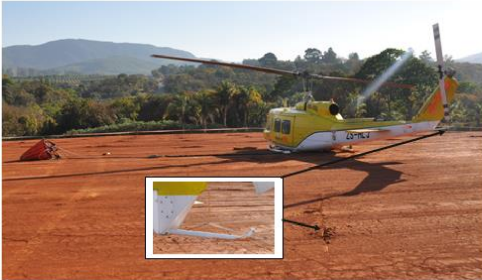
Figure 7: The ground scar mark created by the tail rotor guard during the accident sequence.
