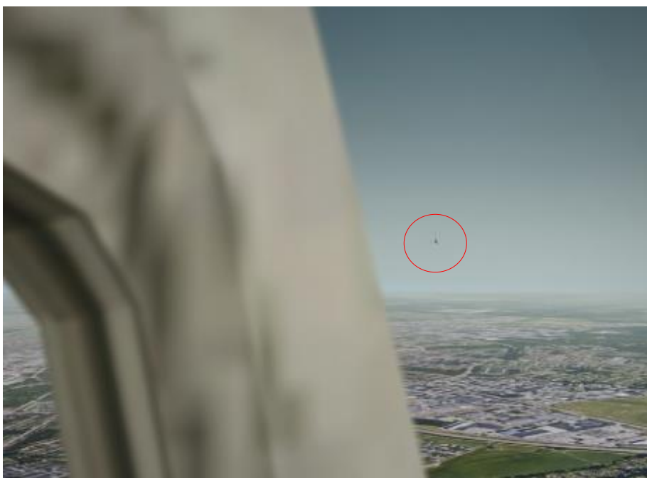
Figure 12. Visualisation of the view from the cockpit of the Cessna just before passing the other aeroplane. The side beam may block the view of oncoming traffic. The silhouette of the PA-28 is seen over the horizon. The red circle marks the PA-28.
