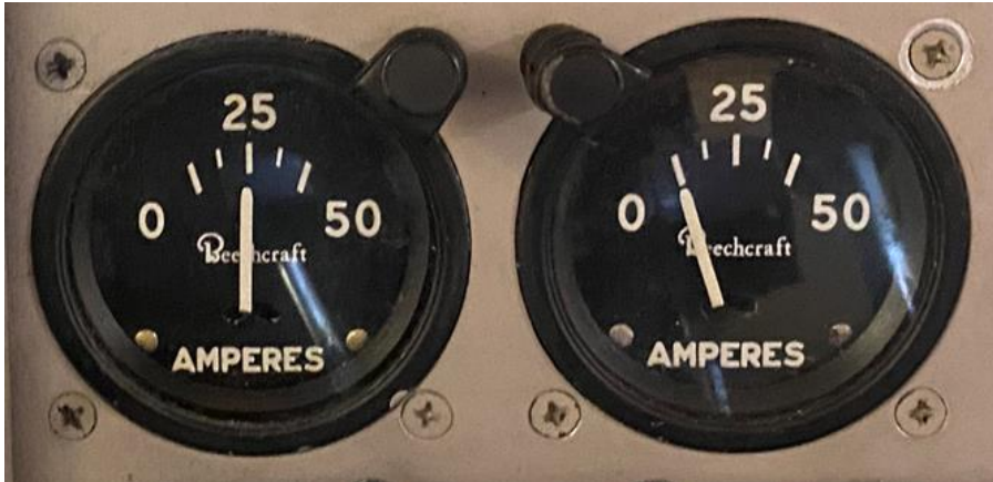
Figure 8. Loadmeters in SE-LUX. The right indicator shows 0 Amperes.
