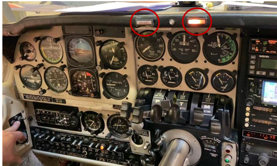
Figure 7. The picture shows left “ALT OUT” light not illuminating when the switch is set to OFF.
