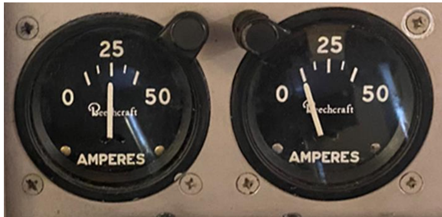
Figure 10. The loadmeters installed in SE-LUX.
