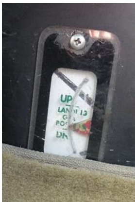
Figure 3. Mechanical nose wheel position indicator.
