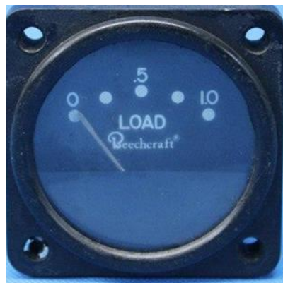
Figure 11. The loadmeter described in the POH of SE-LUX.
