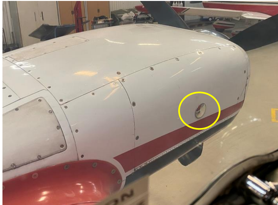
Figure 4. Installed mirror on the left engine cowling to visually verify landing gear position.
