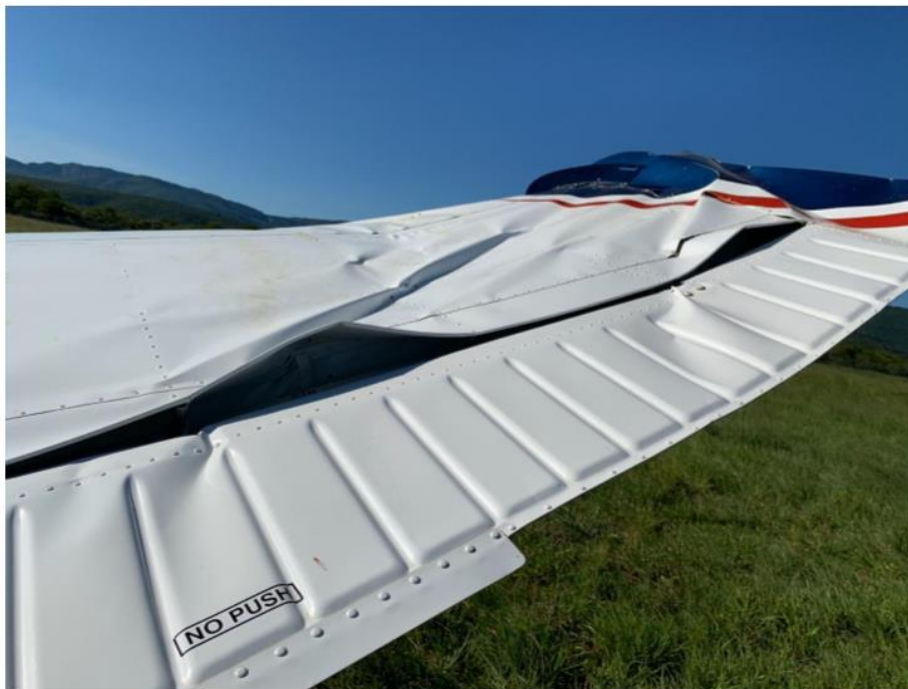
Figure 3: Damage sustained to the aircraft's right wing. (Source: PIC)
