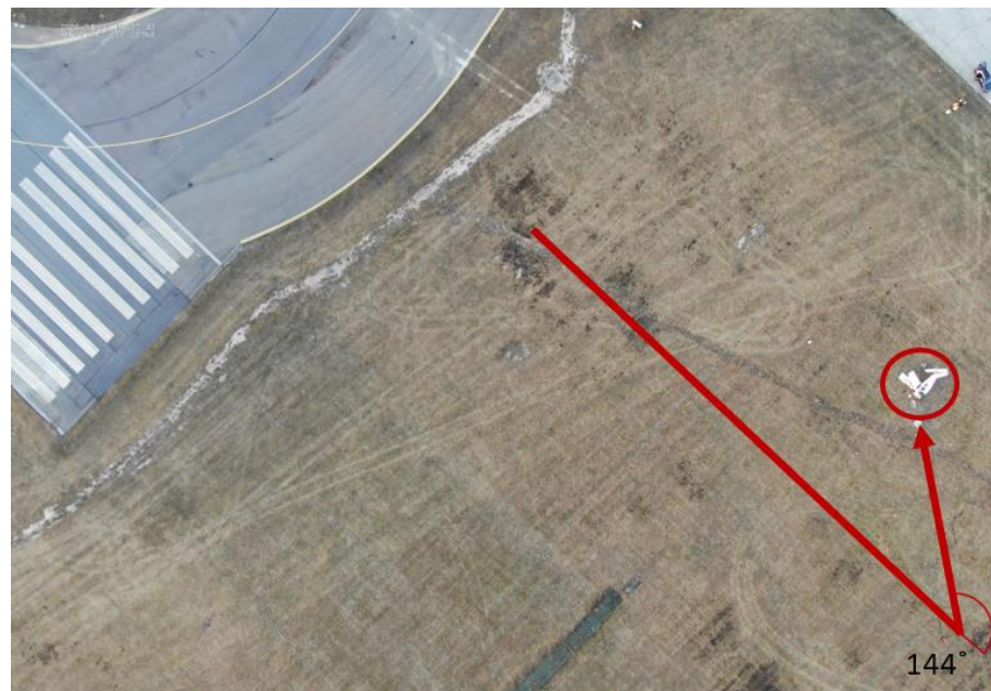
Figure 10. The angle between the take-off heading runway 16 and the impact heading at the time of the accident.
