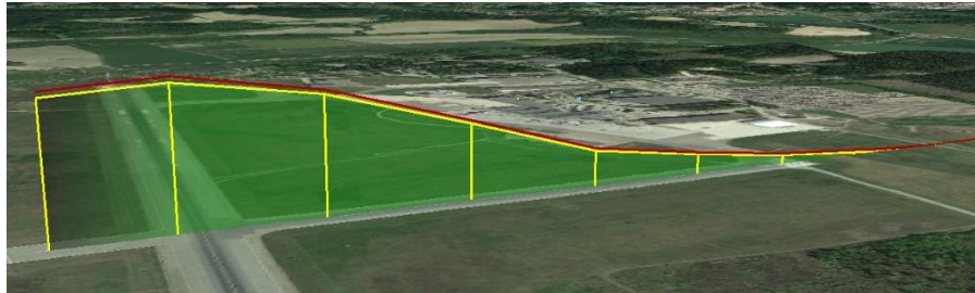
Figure 16. GPS data for glide flight from a simulated engine failure at 300 feet above the runway.
