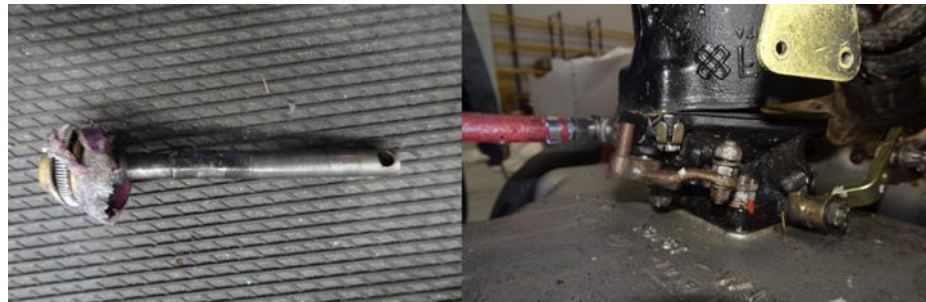
Figure 13. Damaged piston of accelerator pump (left) and part of the carburettor (right).
