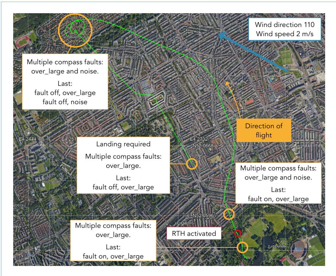
Figure 11: Ground track of the Inspire 2, annotated with the locations of compass errors. (Source map: Google Earth)
