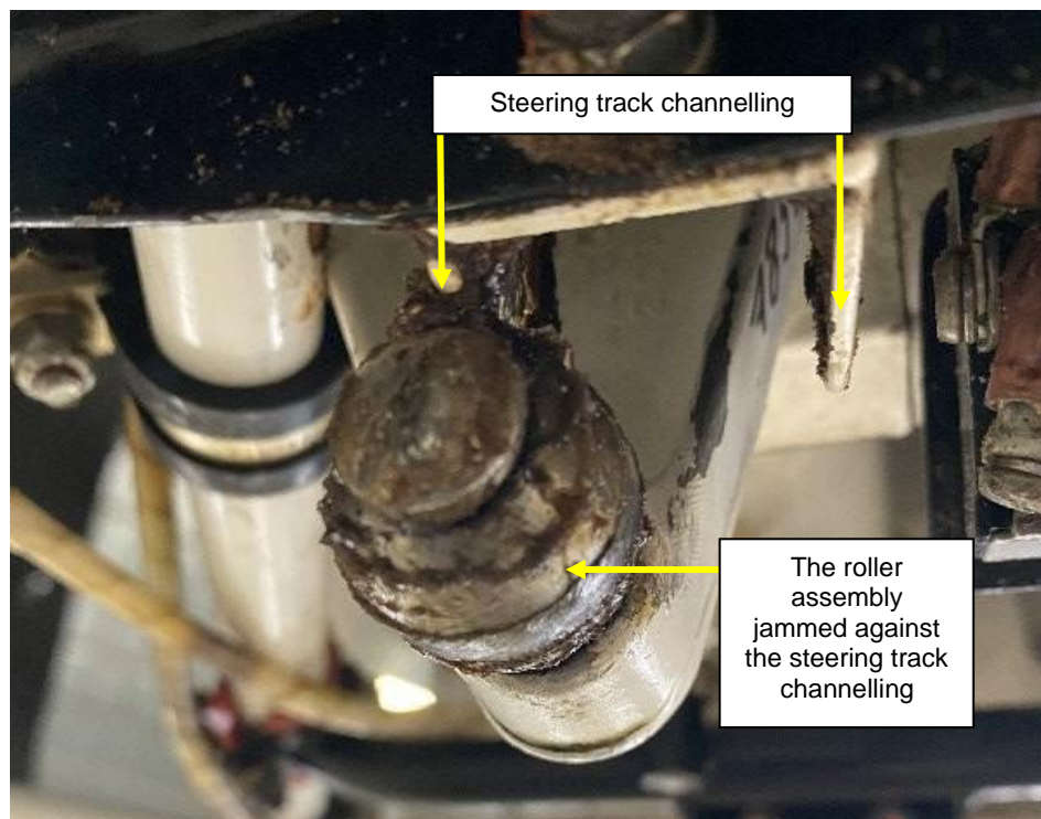
Figure 9: The roller assembly where it had exited the steering track and jammed the nose gear.
