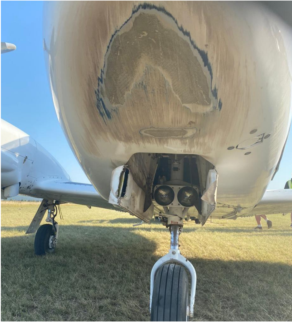
Figure 4: Damage visible to the lower nose cone and nose gear doors. (Photograph courtesy of the AMO)
