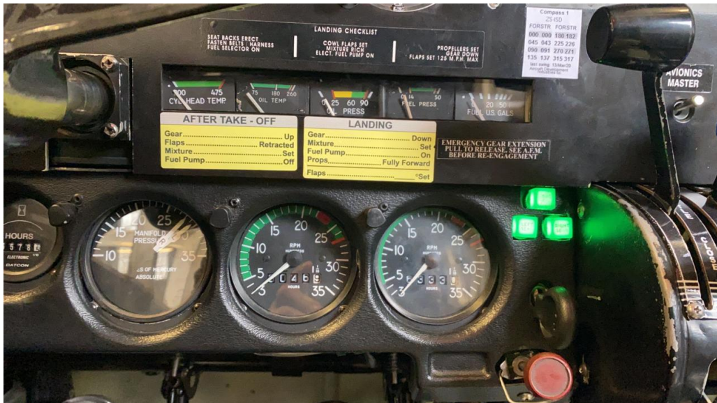
Figure 2: Gear down indication (3 greens) on the instrument panel of ZS-1SD. (Photograph courtesy of the AMO)
