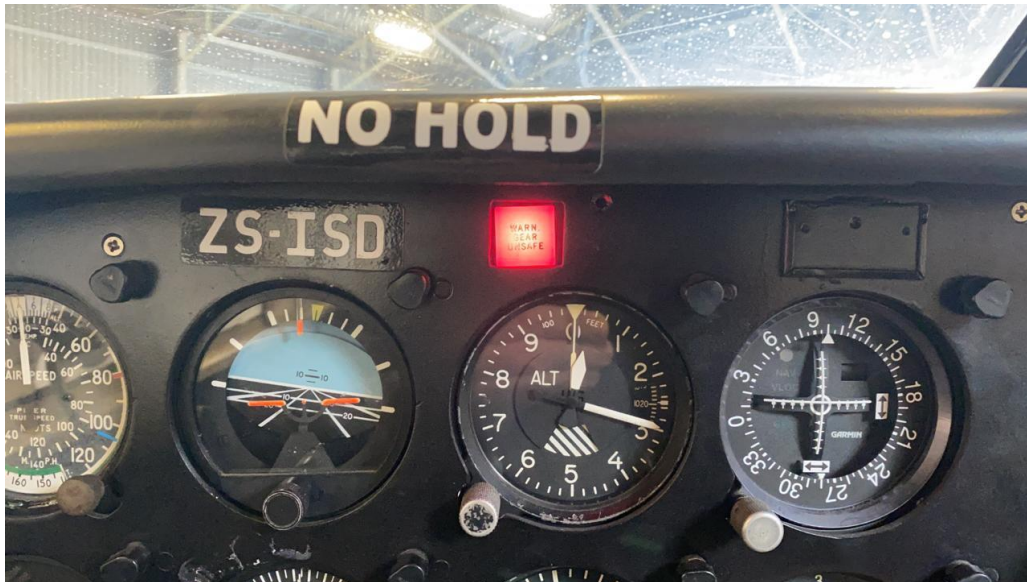
Figure 1: “Warning Gear Unsafe” light on the instrument panel of ZS-1SD. (Photograph courtesy of the AMO)
