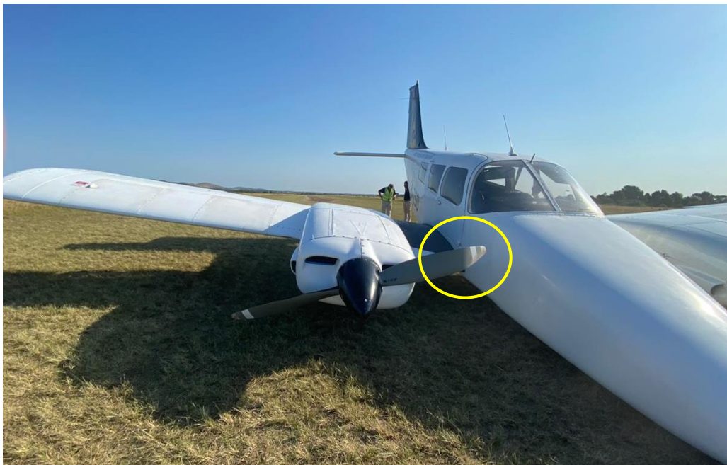
Figure 5: One propeller blade was bent on the right side. (Photograph courtesy of the ATO)
