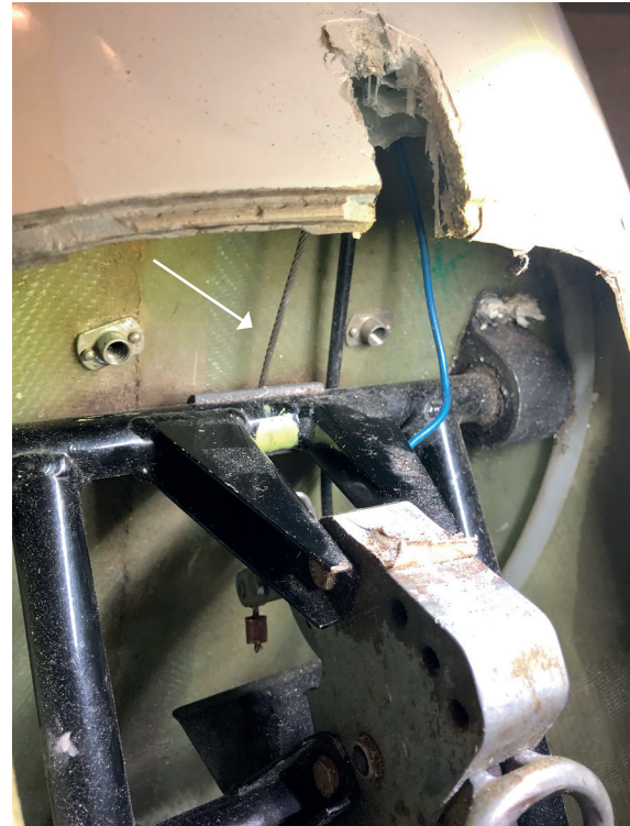
Figure 7: The metal cable of the release mechanism after the routing adjustment. (Source: Dutch Safety Board)
