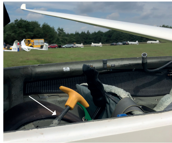
Figure 4: Molded sleeve and yellow release T-shaped handle in another LS8's cockpit. (Source: Dutch Safety Board)
