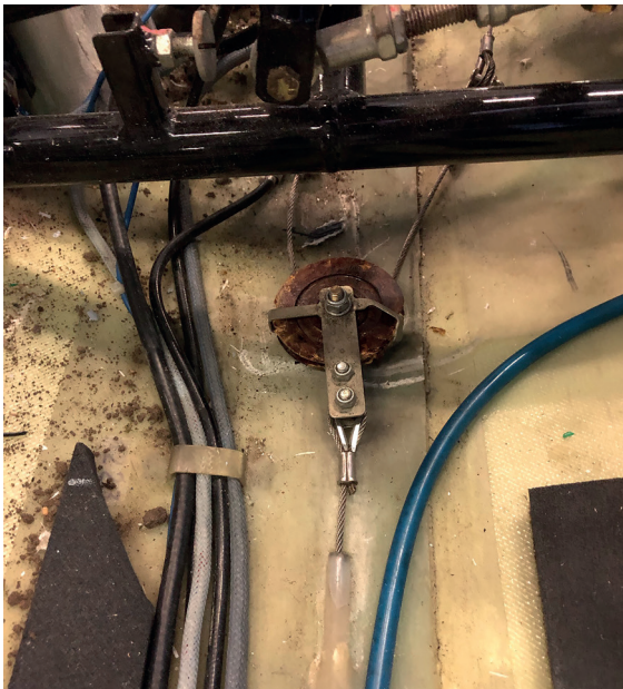
Figure 9: Pulley and release cable at the bottom of the cockpit. (Source: Dutch Safety Board)
