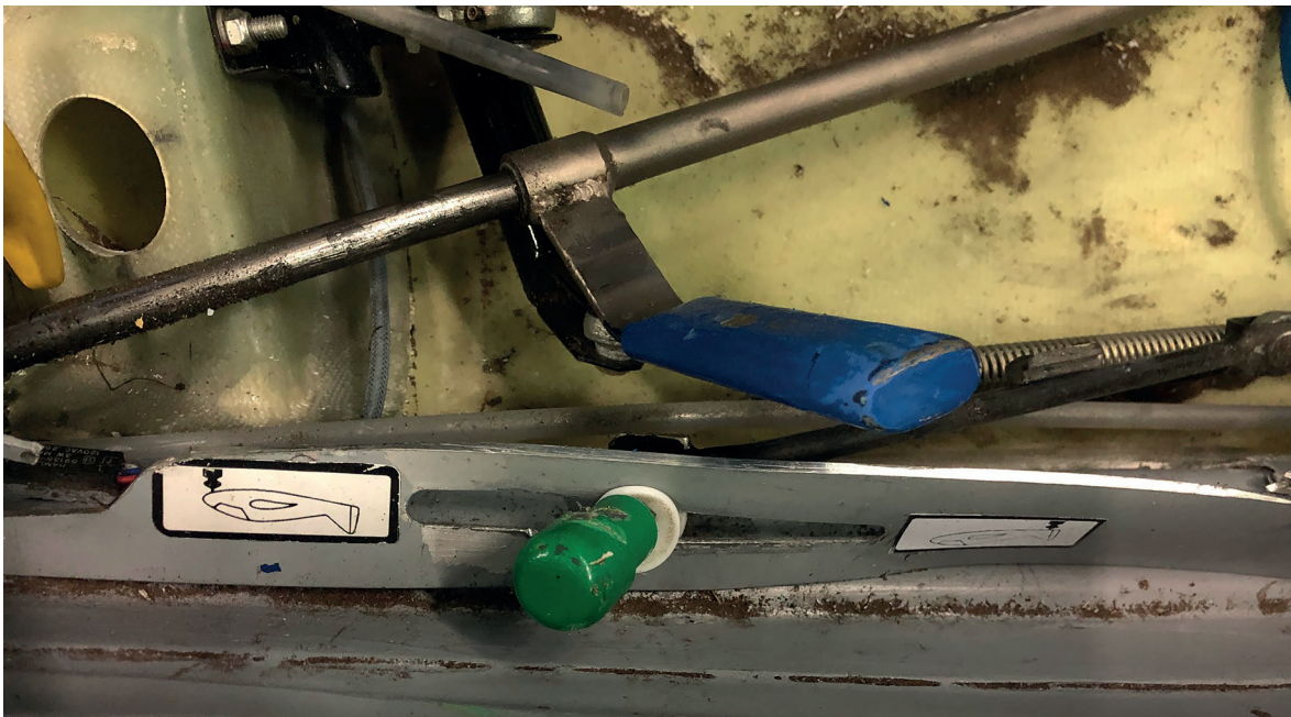
Figure 8: Green trim position indicator and the blue air brake handle. (Source: Dutch Safety Board)
