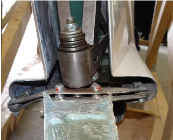
Figure 9. The picture shows the top of the hinge shaft, which consists of an M8 bolt. The rudder is attached to the yoke using the four M6 bolts, two of which are marked in red.
