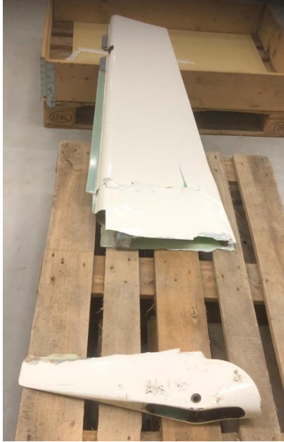
Figure 7. Rudder in two parts. The lower part remained attached to the wreck following the accident.
