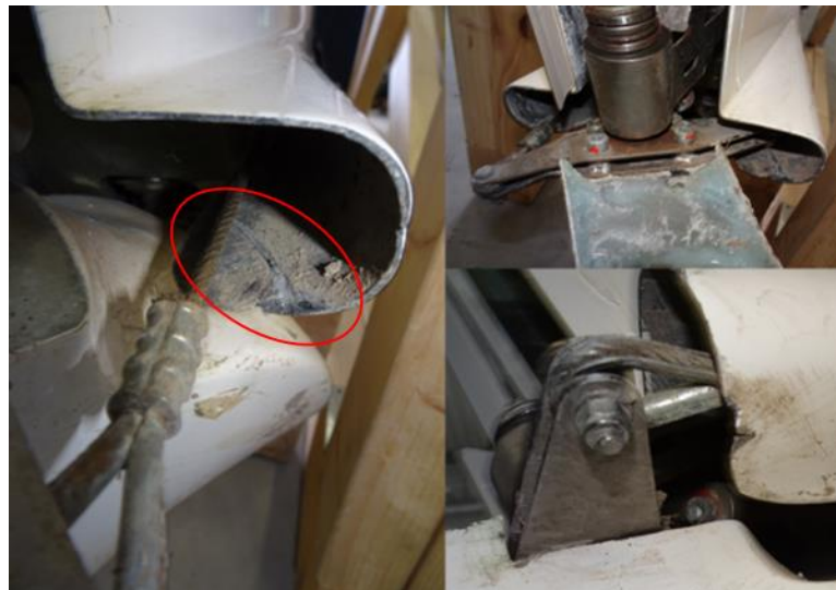
Figure 8. The picture on the left shows a bow-shaped track of wear on the inside of the fairing. The picture on the top right shows the lower rudder hinge. The picture on the bottom right shows the fairing from below.
