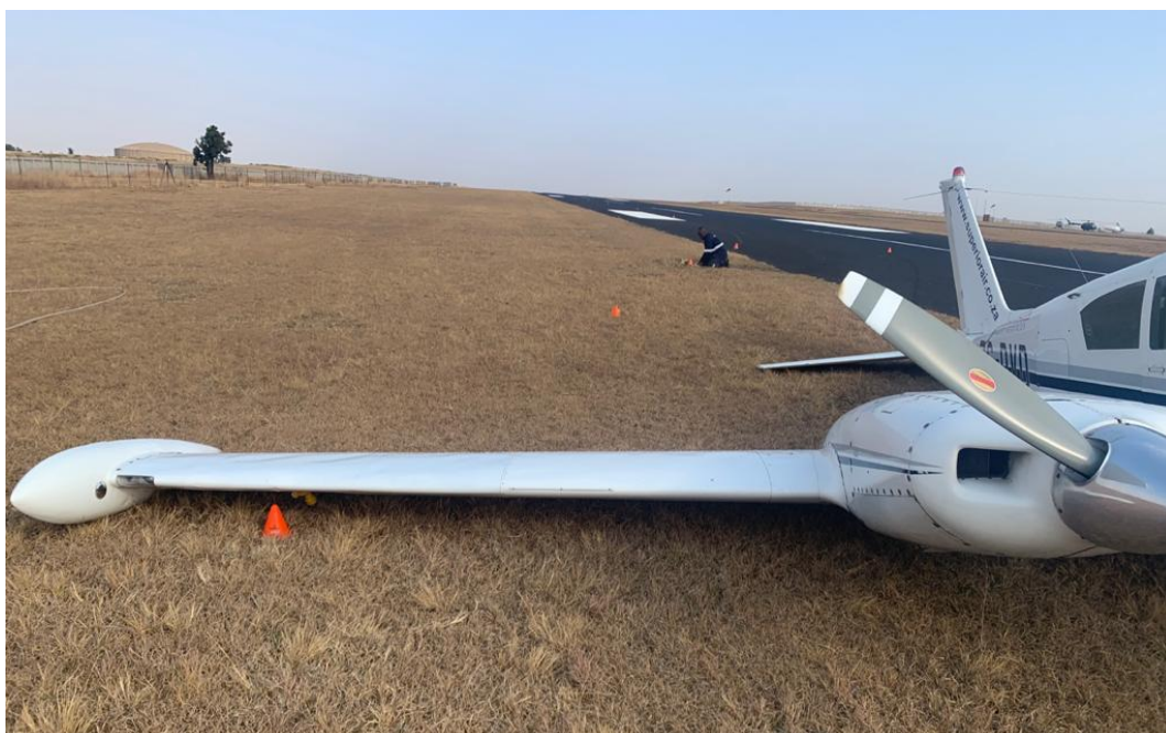
Figure 2: The right-wing tank that came into contact with the ground during the accident sequence.
