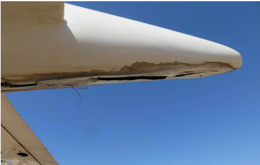
Figure 4: Damage to the lower right-wing tip tank as it scraped along the runway surface.
