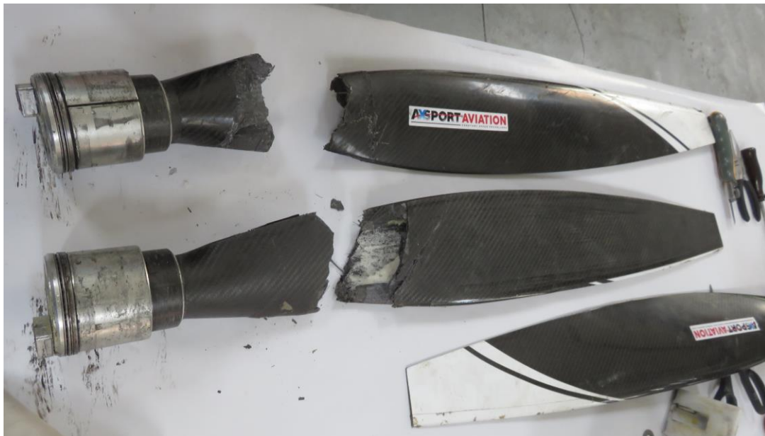
Figure 12: The two blades that fractured during impact.
