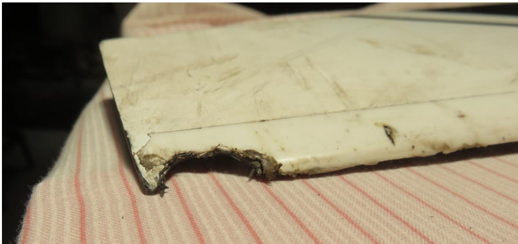
Figure 14: The one blade presented damage on the leading tip.
