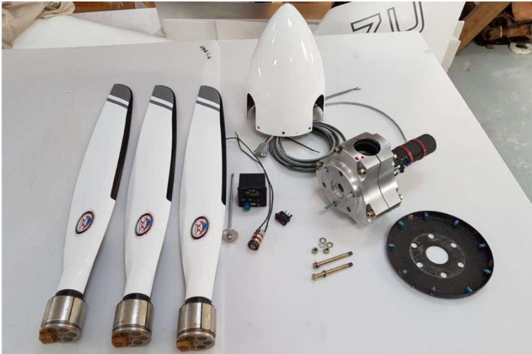
Figure 7: The components of a new propeller assembly. (Source: www.axsportaviation.com ).
