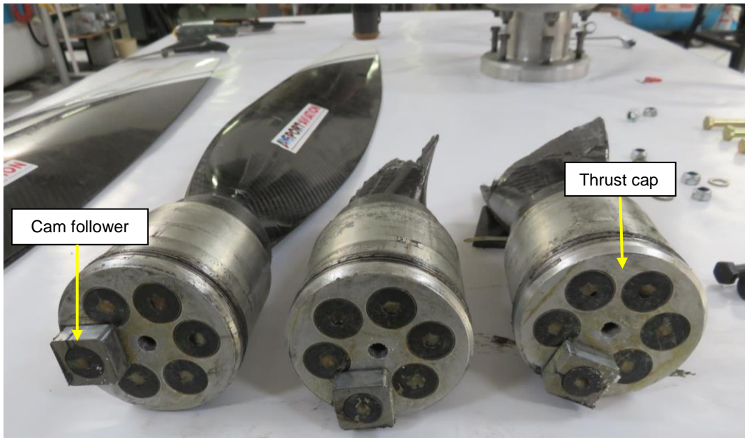
Figure 11: The cam followers and thrust caps of all three propeller blades were secured.
