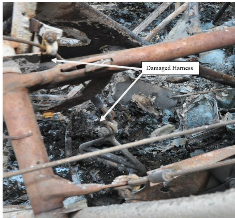
Figure 14: The damaged harness in the wreckage.
