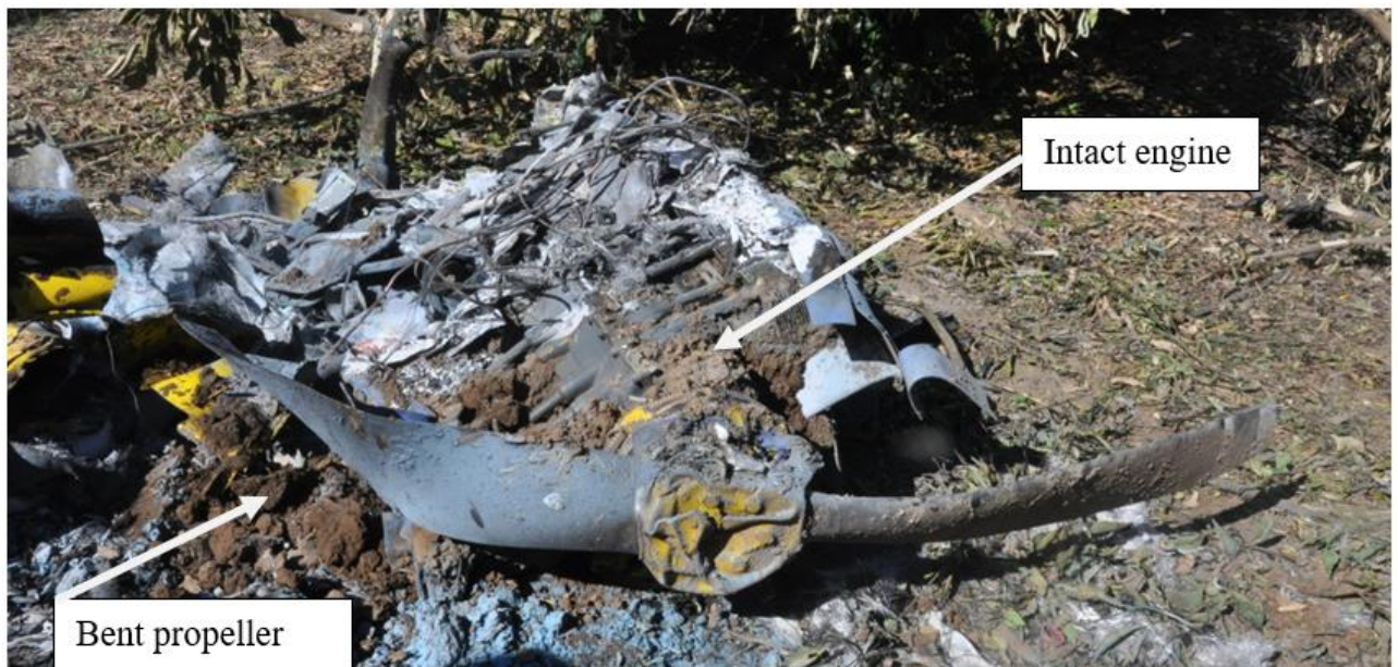
Figure 12: Engine and propeller post-accident indicate that the engine was producing power at time of impact.
