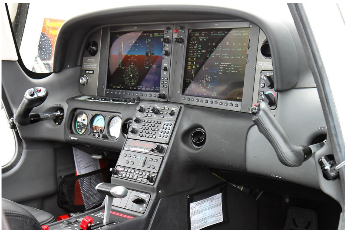
Figure 19: The cockpit layout of the Cirrus SR22 with the side yoke configuration.
