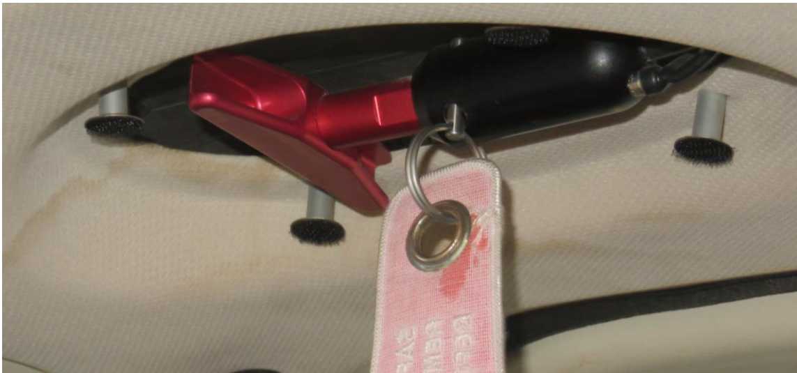
Figure 18: The CAPS handle in the cockpit roof structure.
