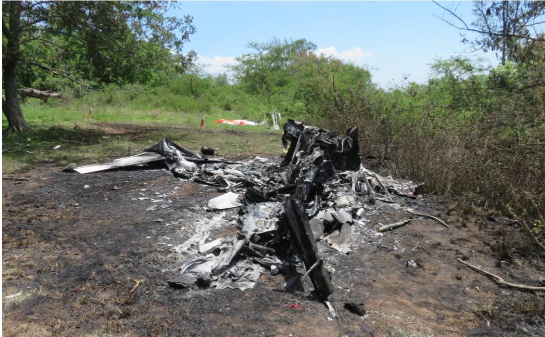
Figure 2: The wreckage was consumed by post-impact fuel-fed fire.
