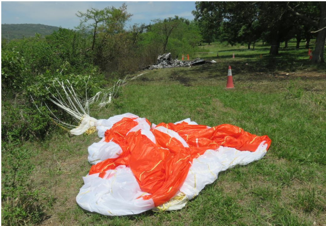
Figure 8: The CAPS was found activated by heat of post-impact fire.
