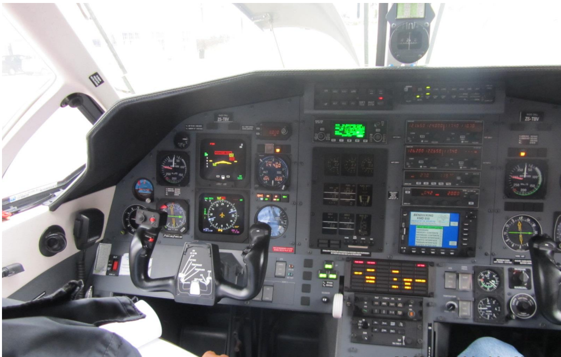
Figure 20: The cockpit layout of a Pilatus PC12 aircraft with a conventional control yoke.
