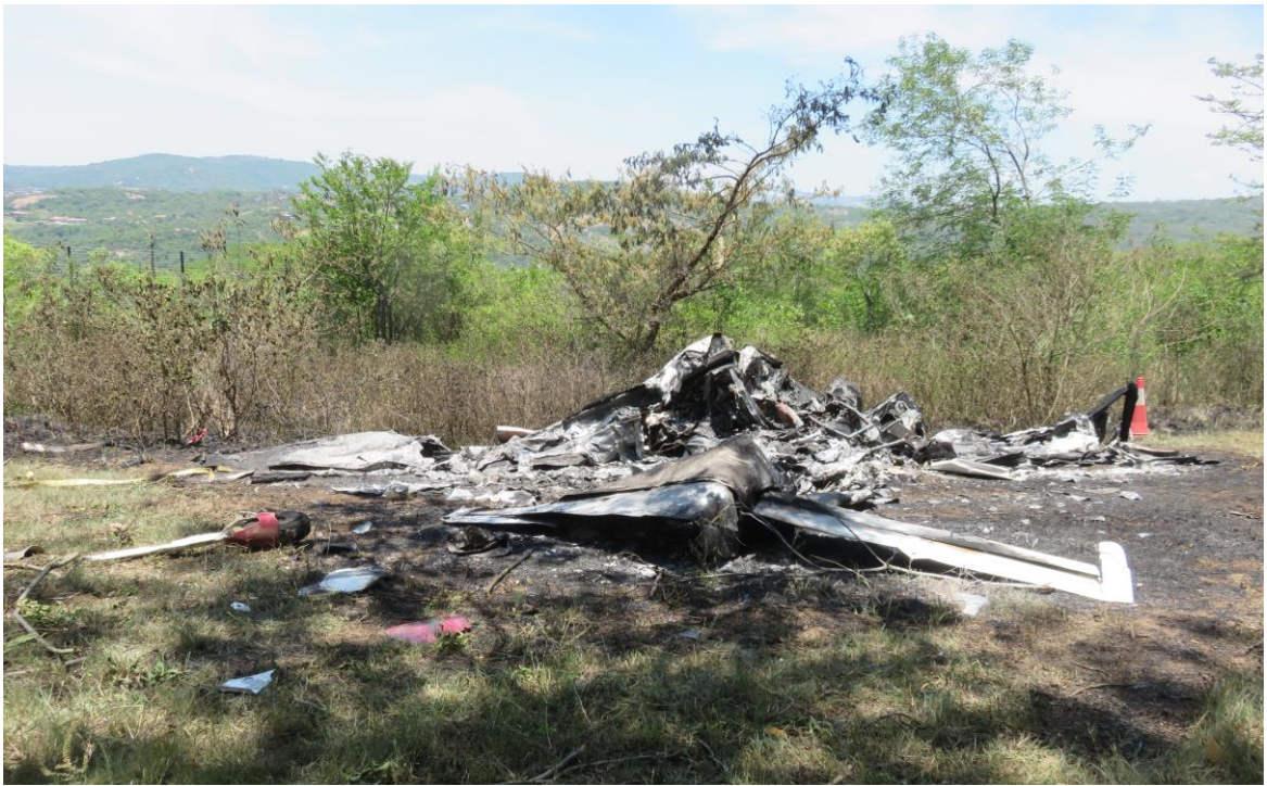
Figure 6: The main wreckage was consumed by post-impact fire.
