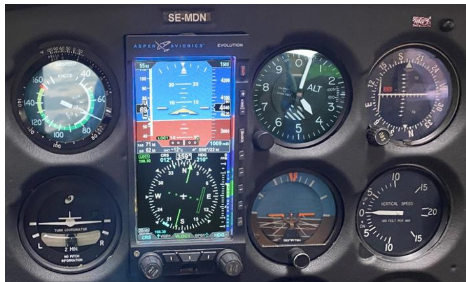
Figure 3. Instrumentation in SE-MDN with Aspen Avionics EFD 1000 as a complement to the primary flight instruments.
