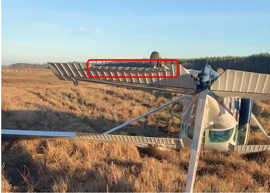
Figure 13. The position of the rudder trim at the accident site. The elevator trim marked by SHK. Photo: Swedish Police.
