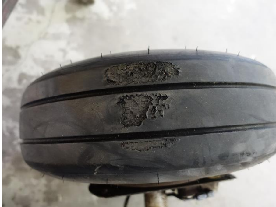
Figure 16. Damage to the left tire of a so-called “Reverted Rubber Hydroplaning”.
