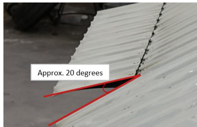
Figure 17. Trim rudder position after the accident.
