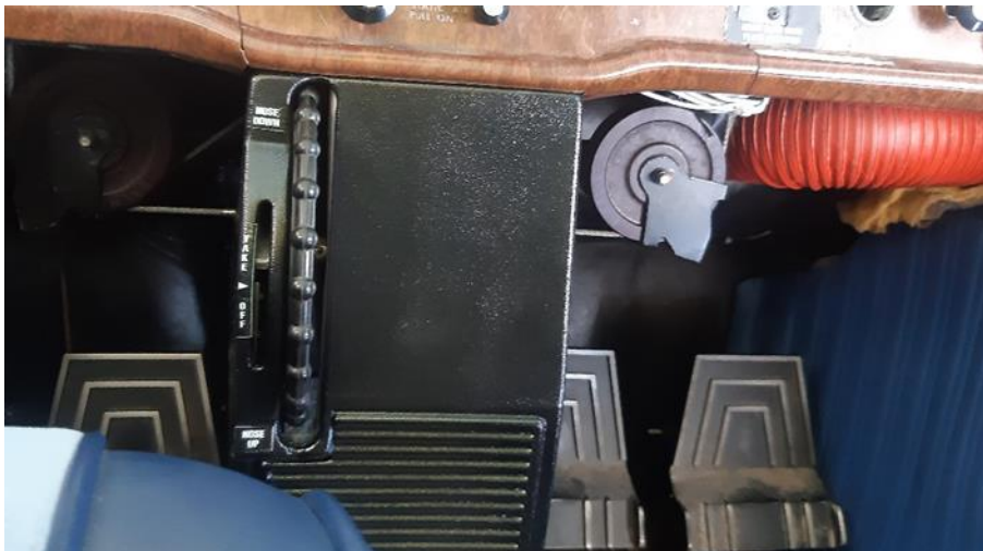
Figure 14. The position of the trim indicator after the accident. Photo: Tord Södergård.
