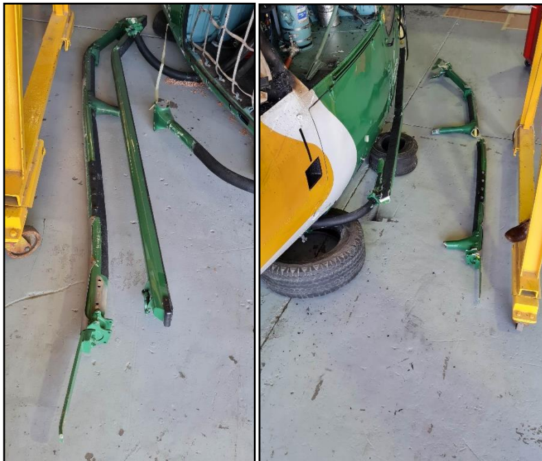
Figure 6: The left skid gears (left image) and the right skid gear (right image).
