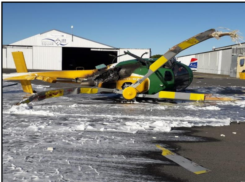
Figure 3: The main rotor blades post-accident.
