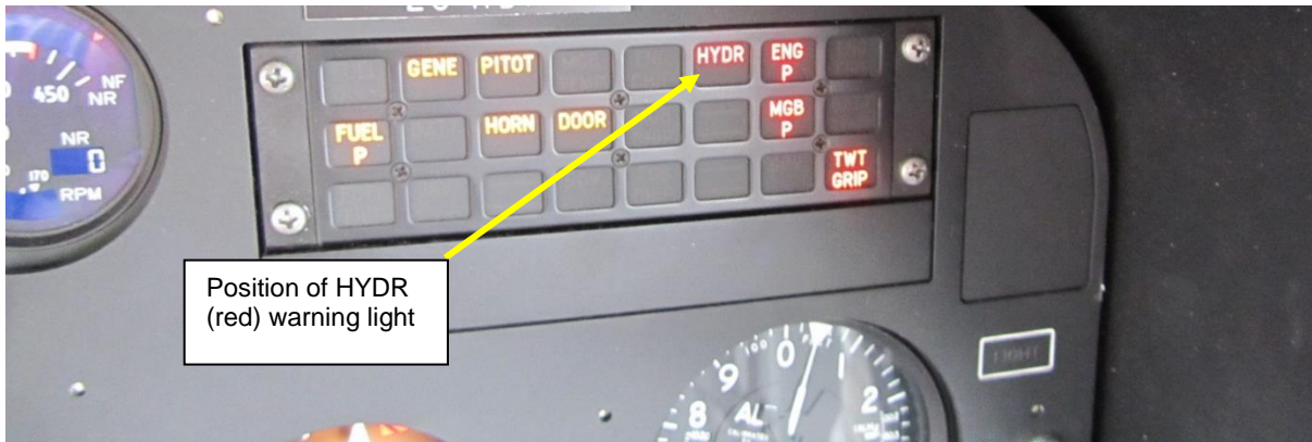
Figure 8: Position of the “HYDR” warning light on the instrument panel.
