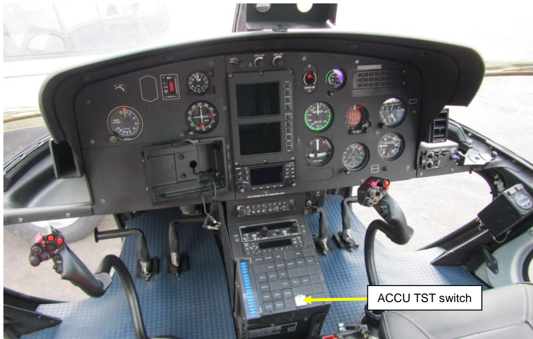
Figure 9: Position of the “ACCU TST” switch on the systems control panel.
