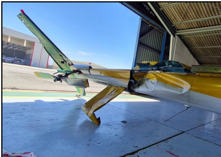
Figure 7: Damaged tail boom and tail rotor.
