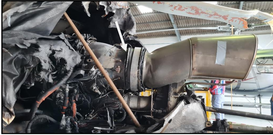
Figure 4: The engine compartment after fire damage.
