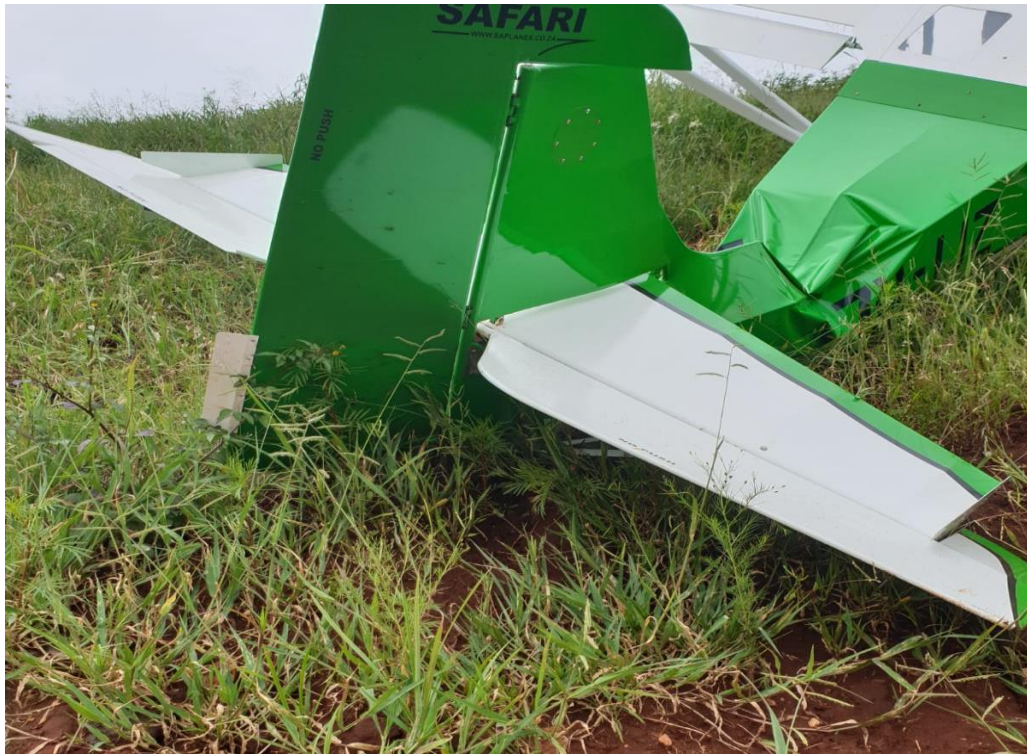
Figure 4: Damage to the tail section.
