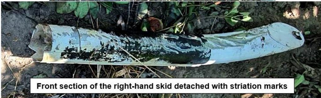
Figure 4: Top image: The left skid attached to the main wreckage. Bottom image: The front section of the right skid showing striation marks.
