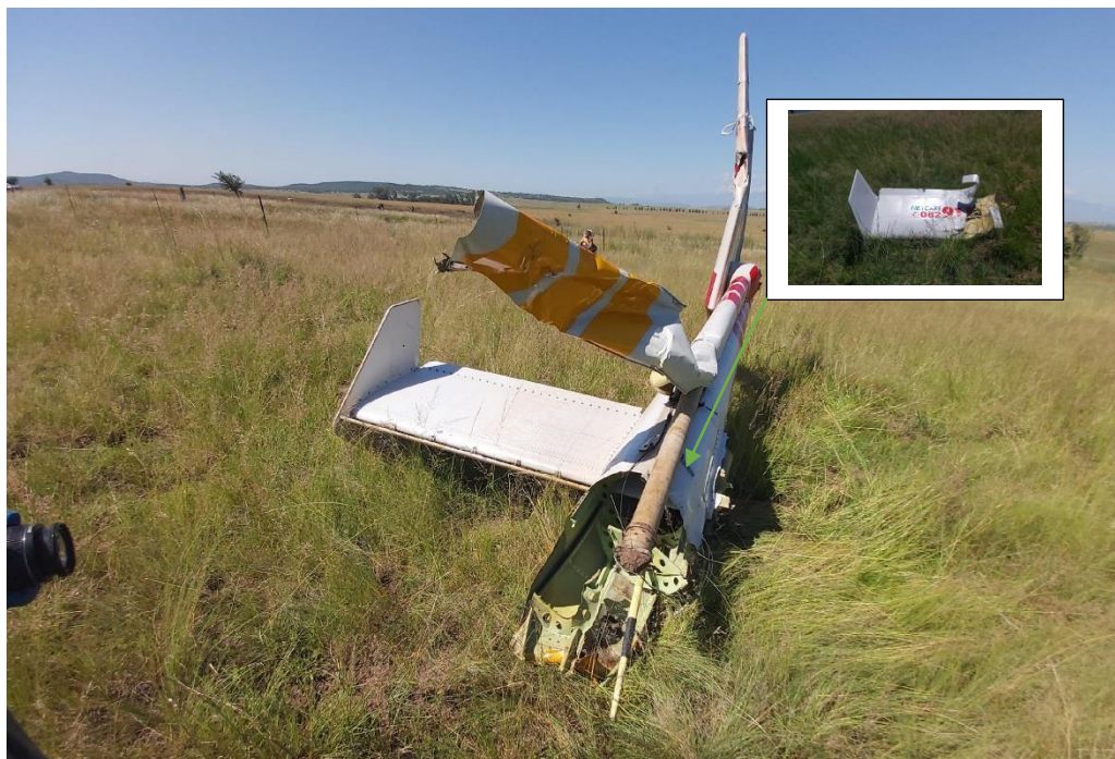
Figure 10: The tail cone assembly repositioned upright was located 129.9m from the main wreckage. (Inset): Left horizontal stabiliser.
