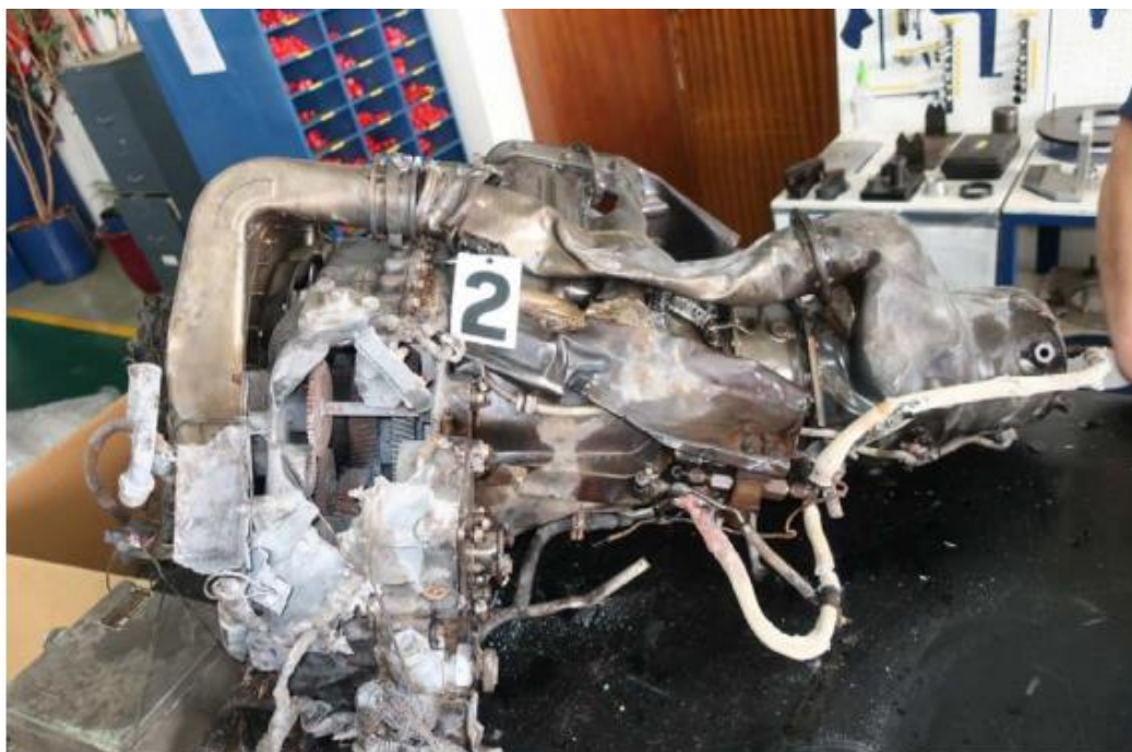
Figure 13: (Engine No.2) As it was recovered.
