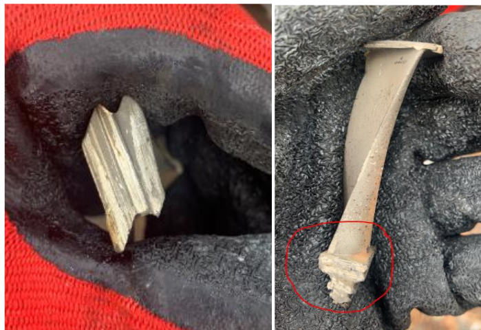
Figure 13: PT Blade shrouded tips.
