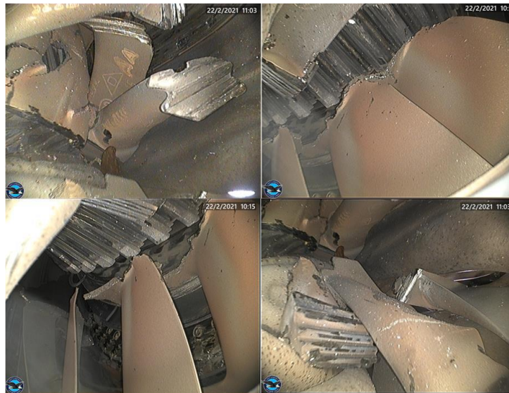
Figure 12: PT blades in the exhaust case.
