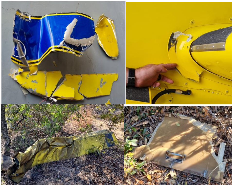
Figure 8: Parts of the left wing tip (top left), left root fairing (top right), right flap (bottom left) and hopper door (bottom right).
