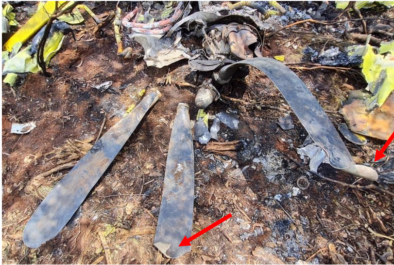
Figure 12: The propeller blades showing rotation signatures on the tips.
