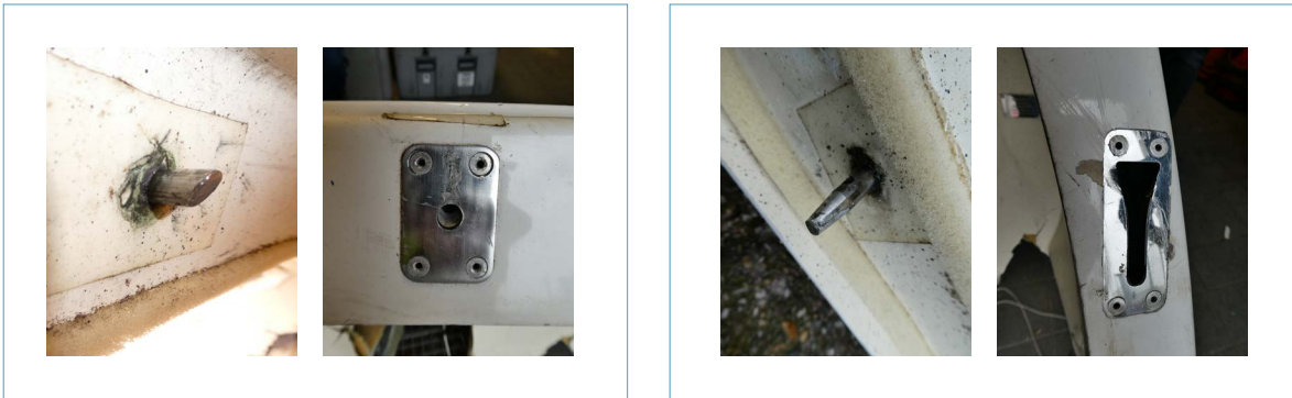
Figure 8a: Locking pin and Figure 8b: Locking socket. (Source: Dutch Safety Board)
