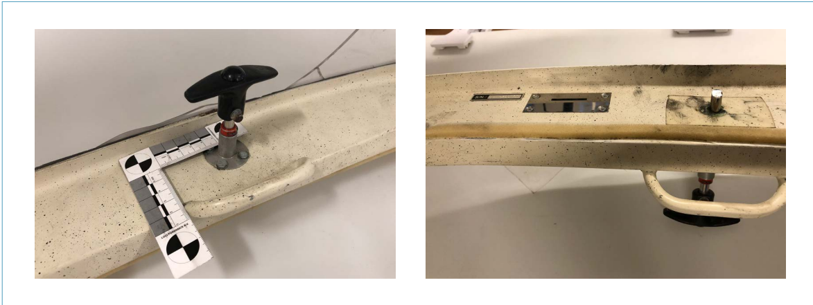
Figures 7a and 7b: Open/closing handle with red ring and locking pin of PH-4E7. (Source: Dutch Safety Board)
