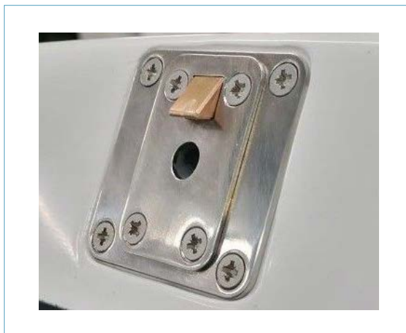
Figure 12: New lock with an additional safety latch. (Source: Aerospool)
