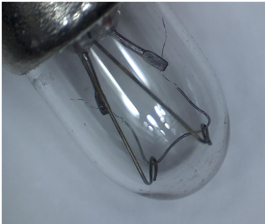
Figure 25. Filament with a normal appearance for comparison. In this case, the warning light for low engine oil pressure.
