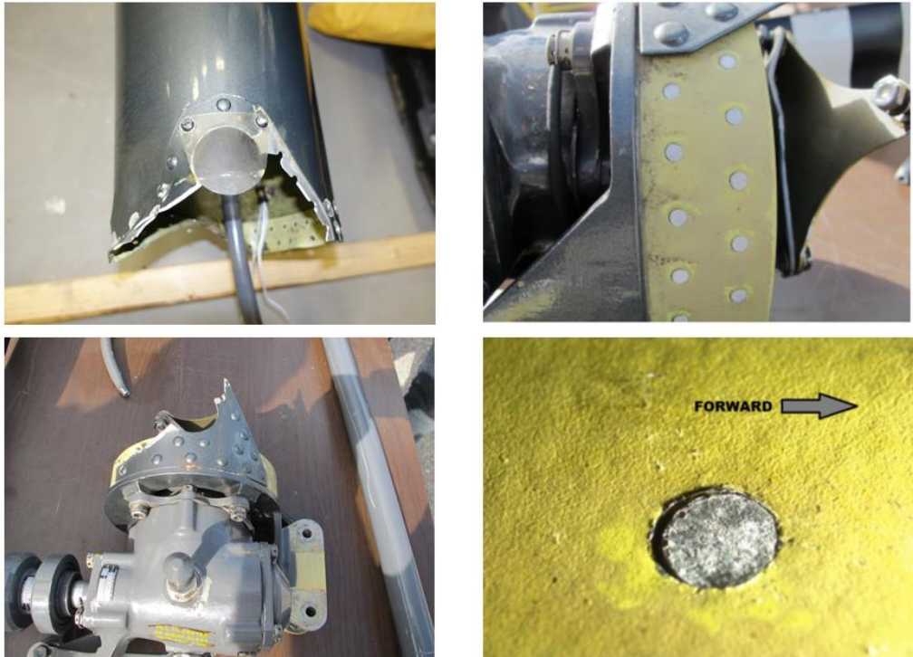
Figure 21. The tail rotor gearbox was broken off the tail boom.
