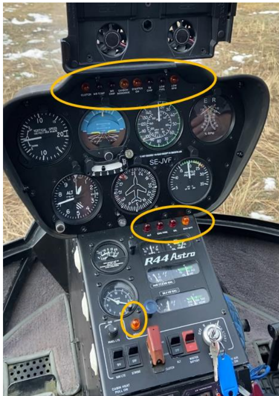
Figure 23. The location of the warning light on the instrument panels. Picture from the start of the flight. Markings by SHK. Photo: Private.
