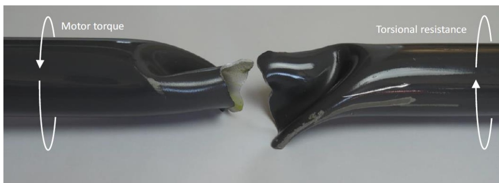
Figure 17. The fracture with load direction.
