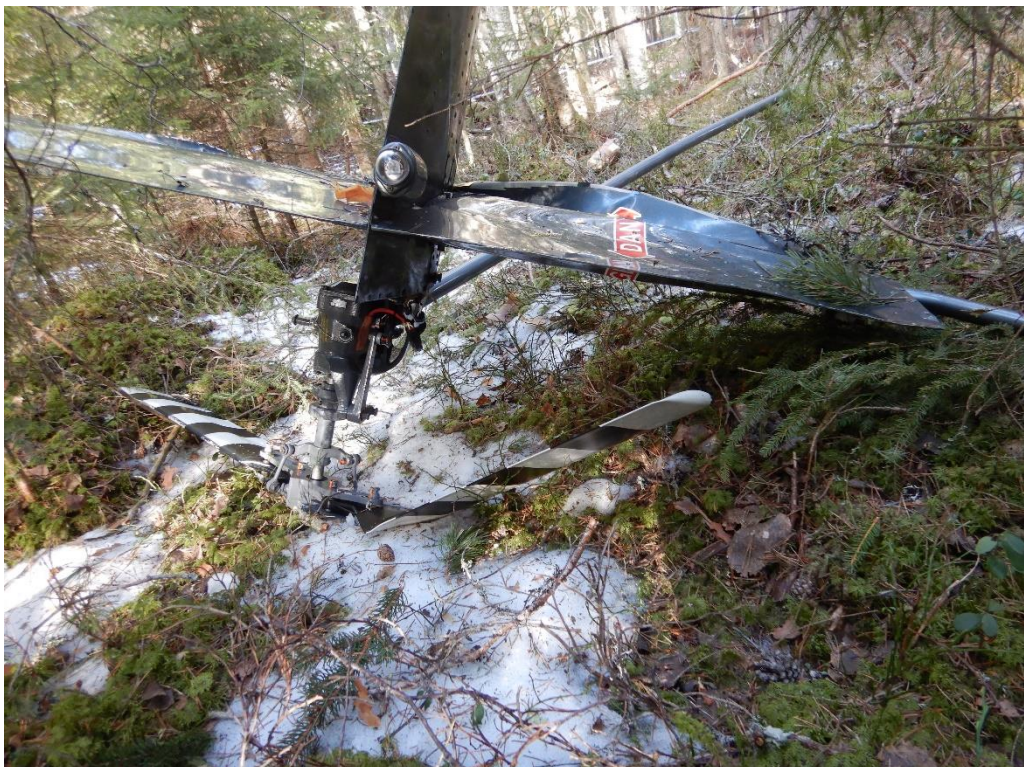
Figure 12. Tail rotor with drive shaft and stabilizer. Damage to the left side of the stabilizer and tail rotor hub.
