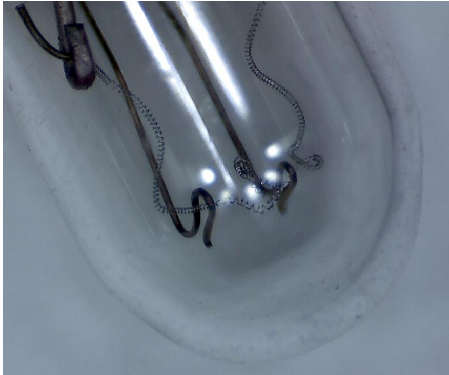
Figure 24. The warning light for low voltage with a stretched filament.
