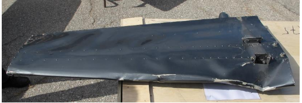
Figure 18. Damage to the horizontal stabilizer.
