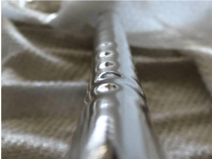
Figure 16. Waveform buckling as a result of torsion.
