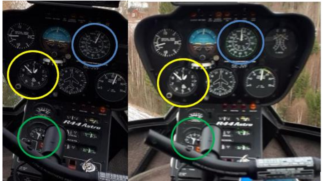
Figure 3. Indicated air speed (blue marking). Altitude (barometric height above sea level in feet, yellow marking) is the same on both occasions. The clock on the instrument panel (green mark) was not set to the correct time. The pictures are cropped by SHK. Photo: Private.
