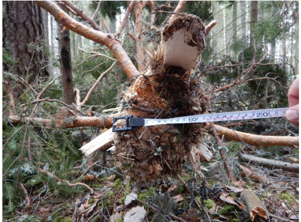
Figure 13. One of the tree trunks that was cut off by the main rotor blades. The diameter of the tree is 13 cm.
