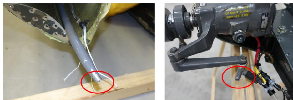
Figure 28. The broken push-pull tube at the tail rotor.
