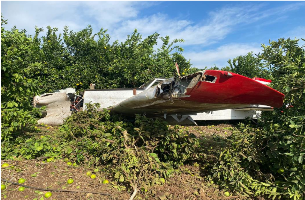
Figure 1: Damage on left-side wing tip.
