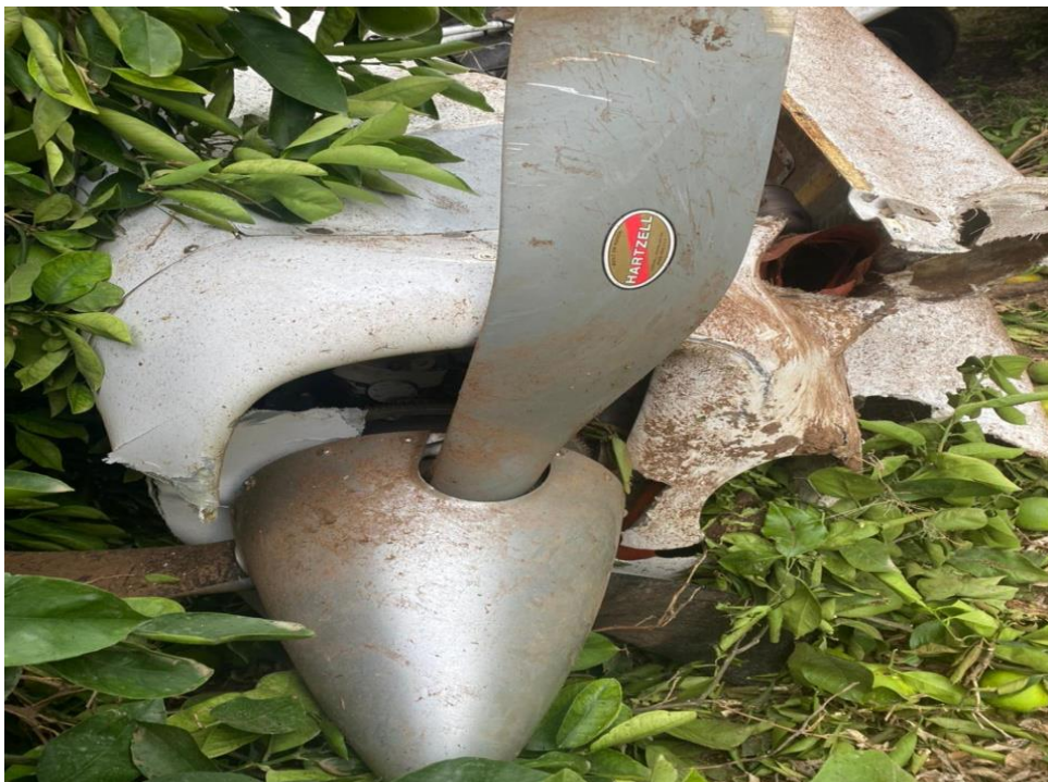
Figure 2: A damaged cowling and bent propeller blades.
