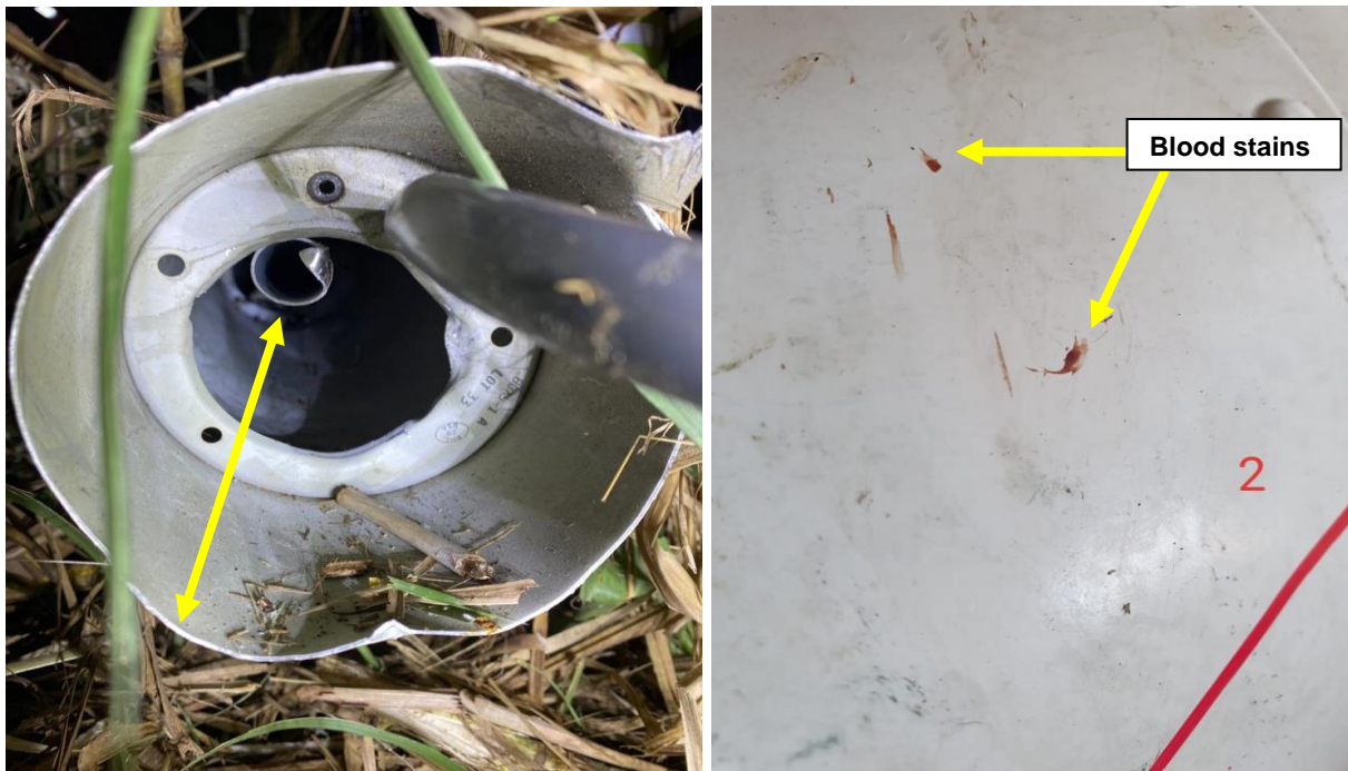
Figures 2 & 3: Left picture shows the tail cone and a fractured tail rotor drive shaft; the right picture shows bird blood stains on the tail cone.
