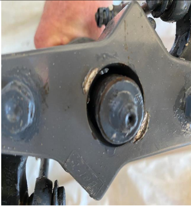
Figures 4 & 5: Left picture shows witness marks left on the tail rotor teetering hinge after a bird strike. Right picture shows bird feathers on the tail rotor blade.
