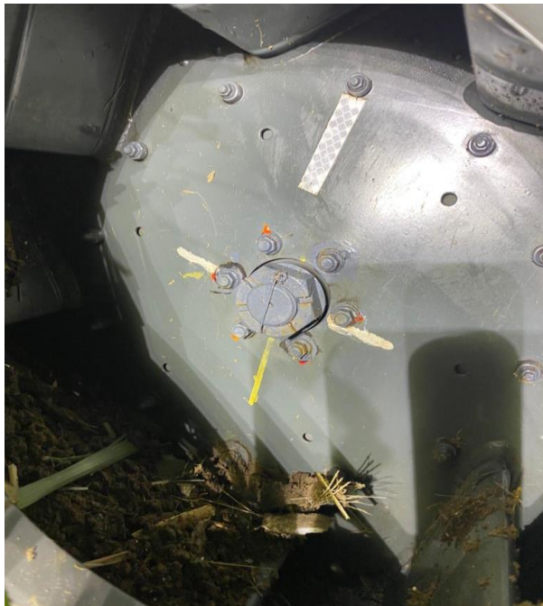
Figures 6 & 7: Left picture shows the engine cooling fan area with misaligned markings on the castellated nut. Right picture shows twist-grip throttle control rod connected to the engine carburettor at maximum power.
