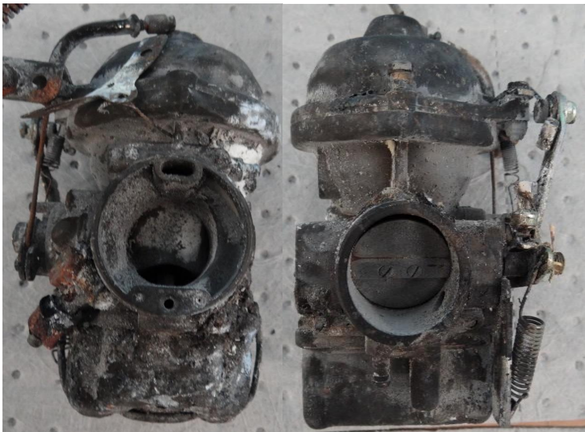
Fig. 8 View of the left carburetor from the throttle and air intake side [source: Institute of Aviation expert opinion].
