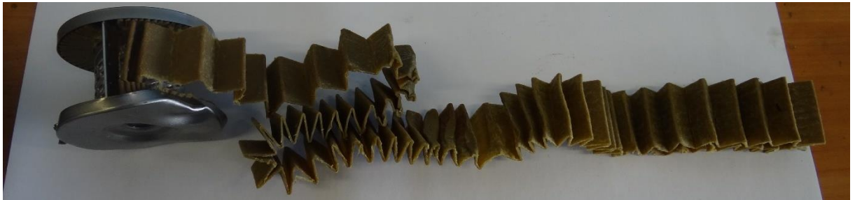
Fig. 21 View of the oil filter cartridge [source: Institute of Aviation expert opinion].
