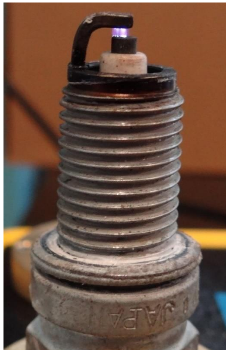
Fig. 15 View of the ignition spark of the lower spark plug in cylinder no. 3 [source: Institute of Aviation expert opinion].
