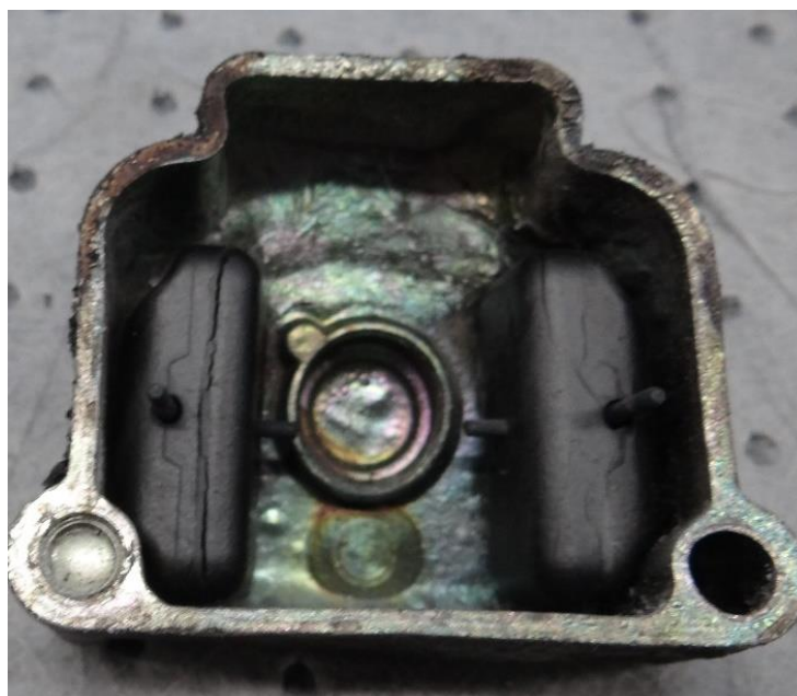
Fig. 9 View of the interior of the float chamber with damaged floats [source: Institute of Aviation expert opinion].
