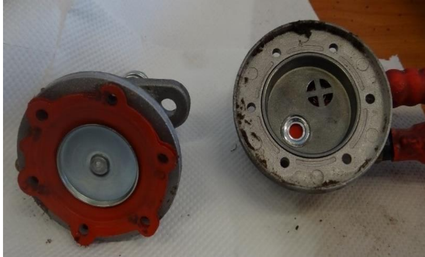
Fig. 14 View of mechanical fuel pump after disassembly [source: Institute of Aviation expert opinion]] After disassembly, no damage to the diaphragm or valves was found (Fig. 14).
