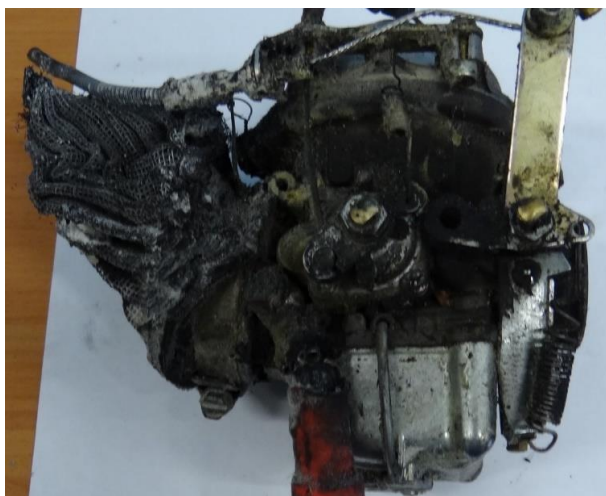
Fig. 11 View of the "right" carburetor from the control side [source: Institute of Aviation expert opinion].
