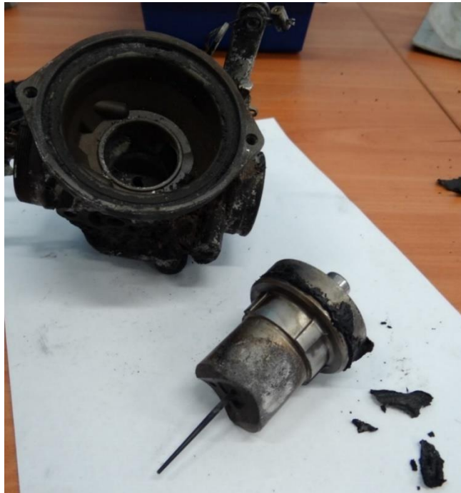
Fig. 10 View of carburetor body and carburetor piston with debris of burnt diaphragm [source: Institute of Aviation expert report].
