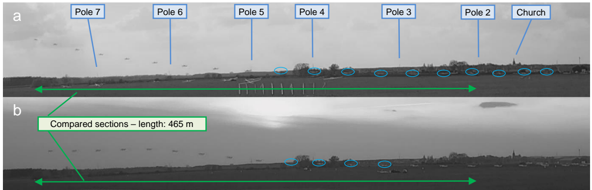
Fig. 30 The airplane positions at 1 s intervals on videos from the camera at EPLS [source: Google Earth, airplane take-off recordings].
