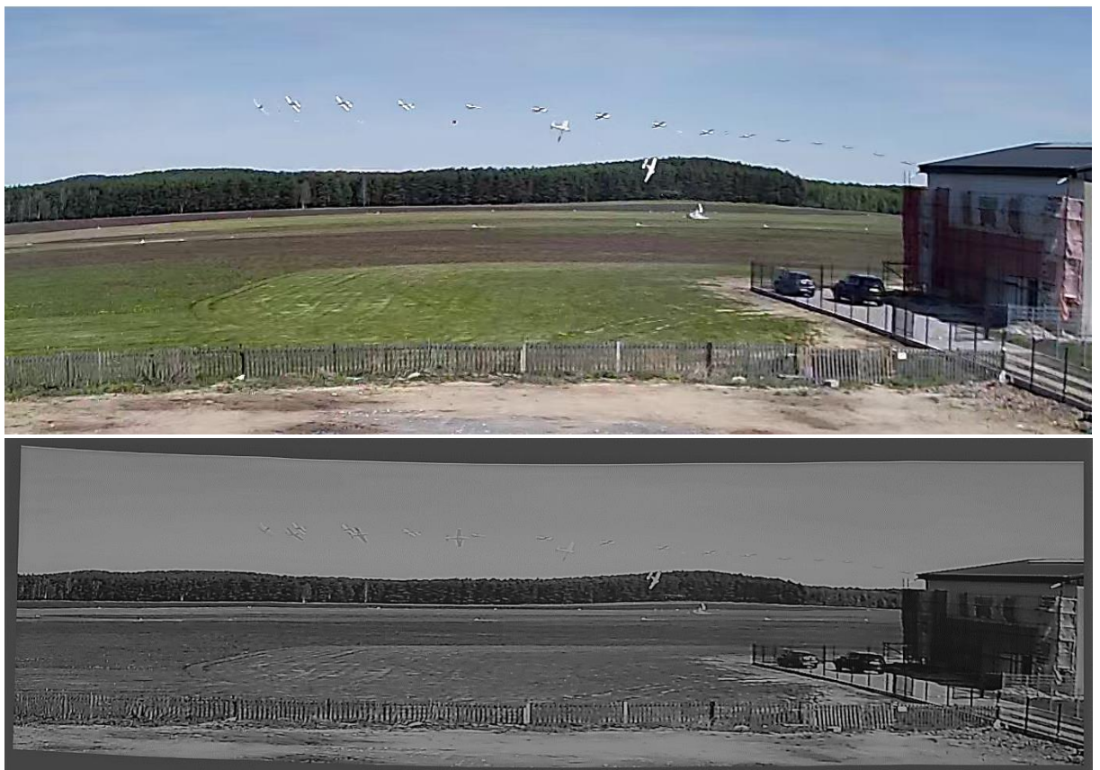
Fig. 25 Airplane positions at 1 s intervals based on the recording from the house on the outskirts of the aerodrome - original (top) and after geometry correction (bottom) [source: PKBWL analysis].
