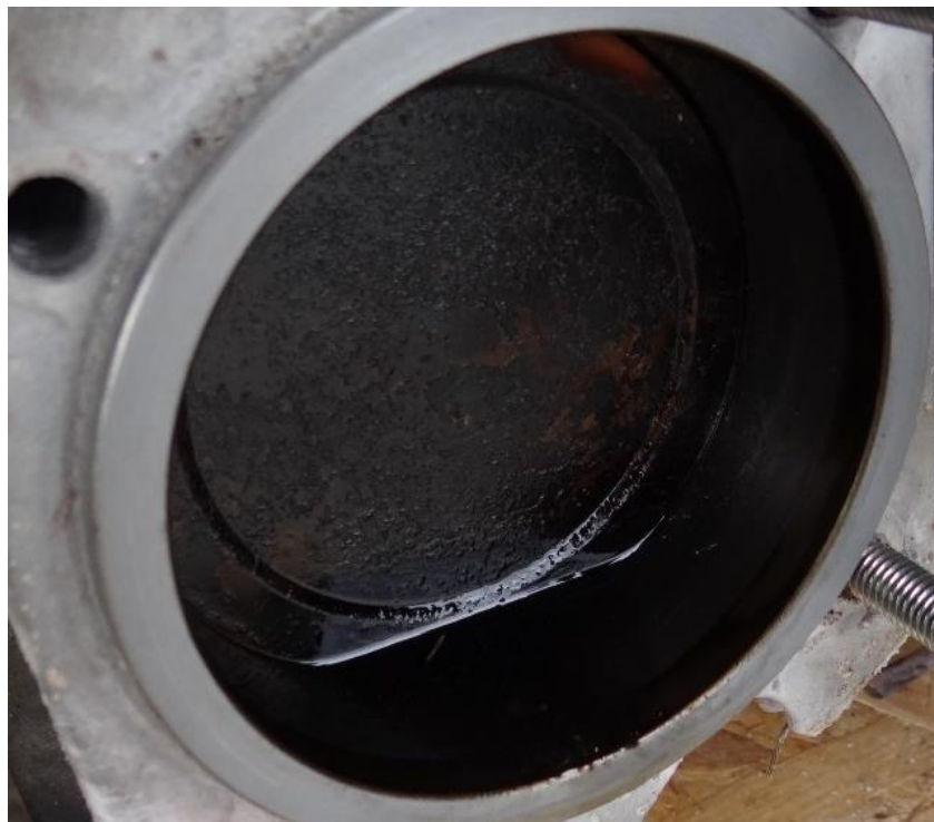
Fig. 20 View of cylinder and piston crown of cylinder no. 2 [source: Institute of Aviation expert opinion].
