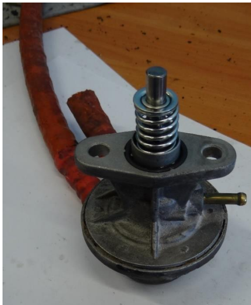
Fig. 13 General view of the mechanical fuel pump [source: Institute of Aviation expert opinion]]
