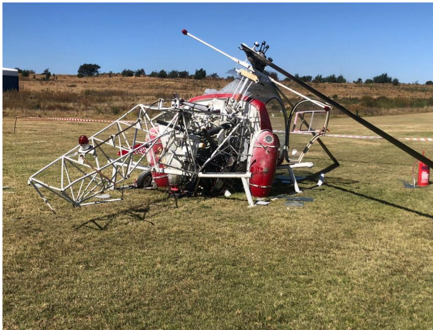
Figure 2: The helicopter's tail boom with the severed tail rotor. (Source: Pilot)
