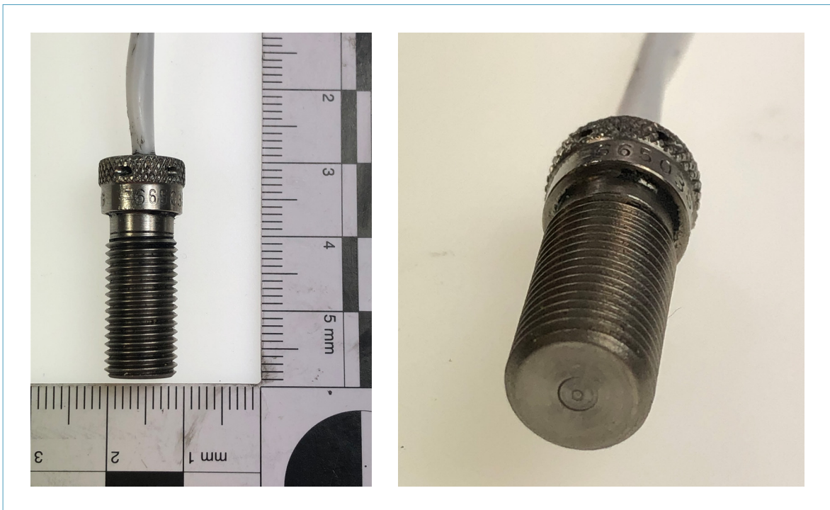
Figure 3a and 3b: Magnetic pick-up in its original state. (Source: Dutch Safety Board)
