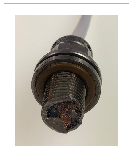
Figure 10: Damaged magnetic pick-up. (Source: Dutch Safety Board)
