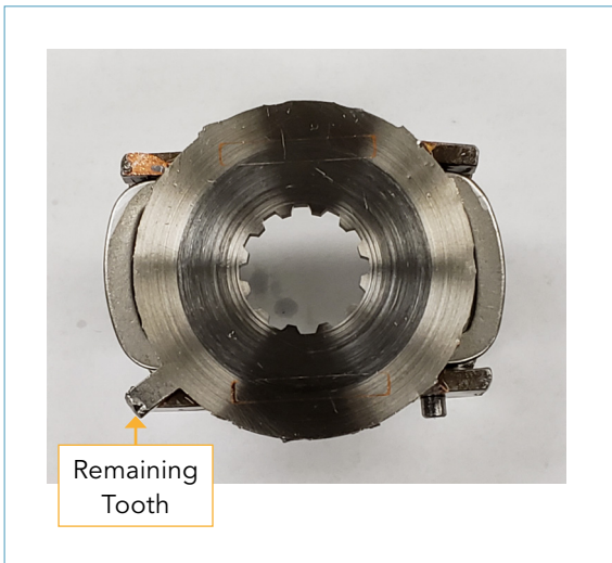
Figure 13: Bottom view of damaged ballhead assembly. (Source: Woodward)
