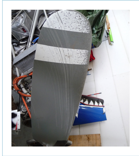
Figure 8: Spanwise damage on prop blade. (Source: Dutch Safety Board)
