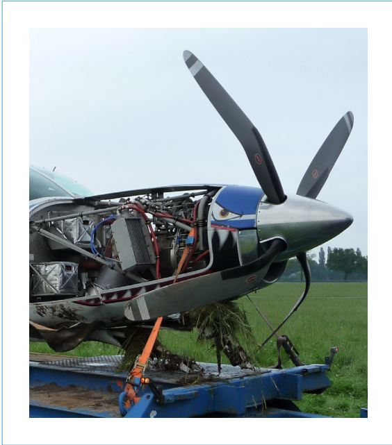
Figure 7: Propeller blade damage. (Source: Dutch Safety Board)
