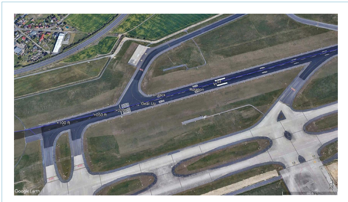
Figure 6: Relevant data of the takeoff projected on Runway 25R. (Source: the operator)
