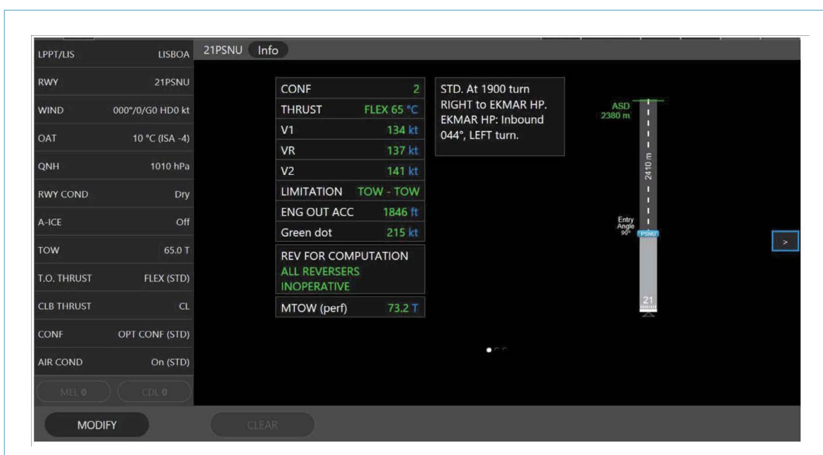
Figure 9: New software calculation display for Runway 21 Position U of Lisbon Airport. (Source: AAIB)
