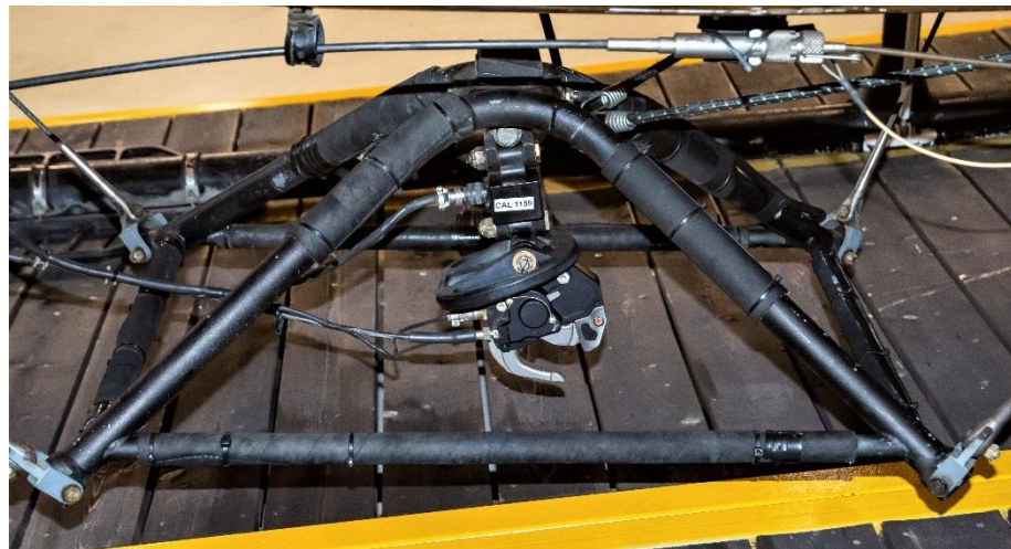
Figure 2. Sling load equipment with a cargo hook.
