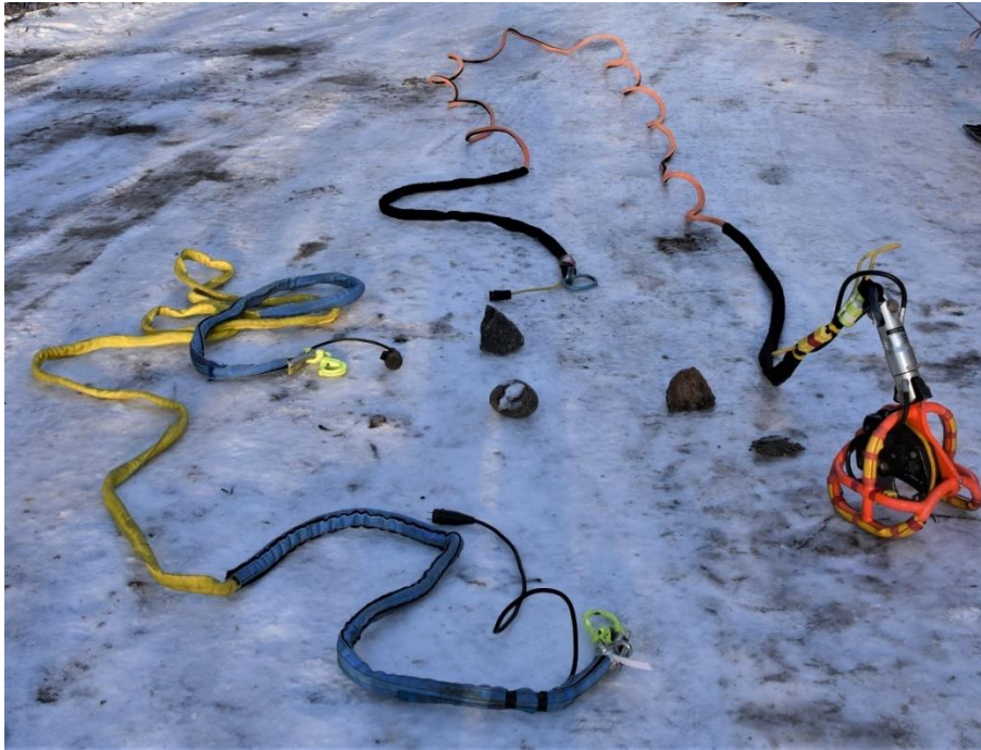
Figure 3. The sling with a lower hook (on the right) and the 10-metre-long extension sling.
