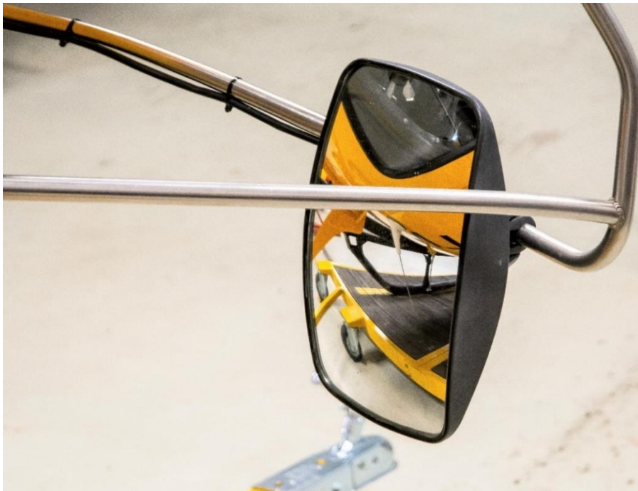
Figure 7. Electrically heated rear-view mirror.
