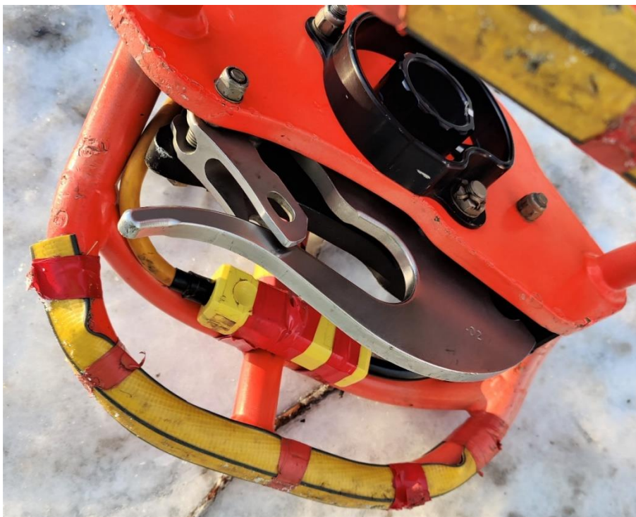
Figure 4. Close-up image of the lower hook.
