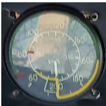
Fig. 6. Airspeed indicator (ASI) installed on SP-STYL aircraft (green arc up to V = 160 kph., yellow arc up to V=230 kph, red line at V_{NE} \cong 250 kph.) and the table of ASI marking as per Flight Manual [source: SCAAI]
