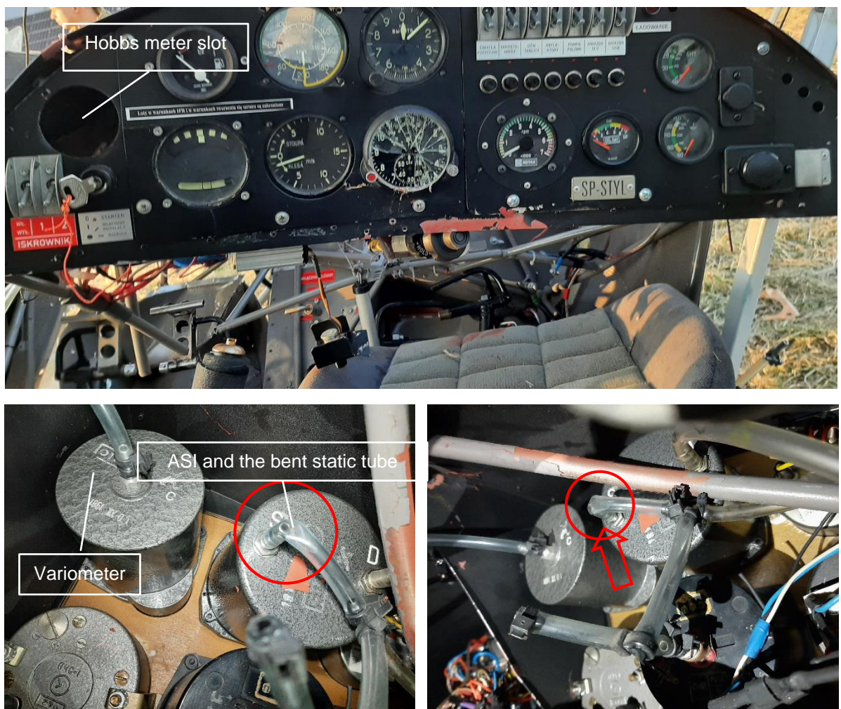
Fig. 5. Avionics of SP-STYL a/c and static pressure tube connected to ASI [source: SCAA]
