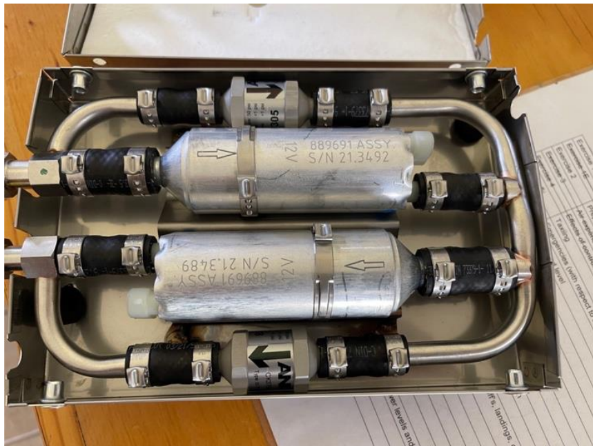
Figure 4: Serviceable fuel pump assembly, similar to the one that was fitted on the accident aircraft. (Source: AMO)
