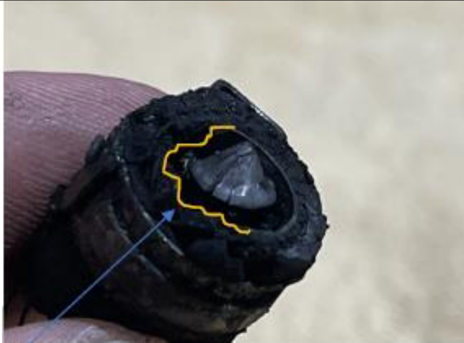
Figure 6: Fuel outlet nipple in the auxiliary pump showing a cracked area, and the yellow line indicates the deformation of the nipple housing. (Source: AMO)
