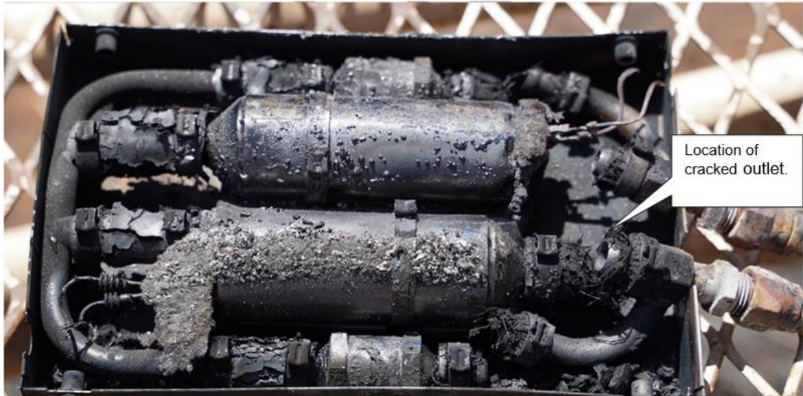
Figure 5: Opened fuel pump assembly at the accident site - SN 19.5057 (Source: AMO)
