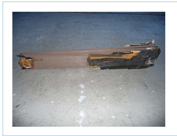
Figure 6: Parts of hull structure frames. (Source: Dutch Safety Board)
