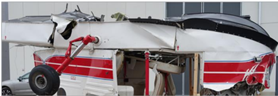
Figure 24. Left side of bottom hull, keel, nose and cabin. The fuselage is upside down in the picture.
