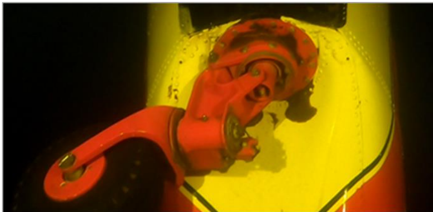
Figure 21. The position of the Tail Wheel during the diving. Photo: The Swedish Police.
