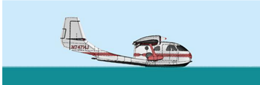
Figure 29. The hull of the aircraft contacts the water surface without the step breaking the water surface.
