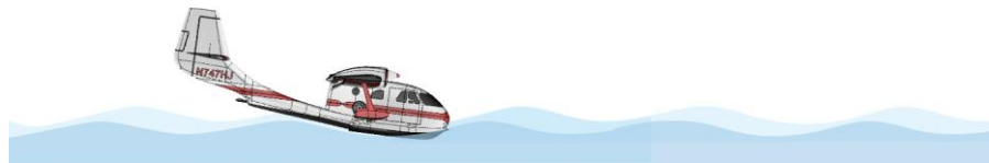
Figure 32. Principle sketch, the aircraft tips forward and the nose is pushed into the water.
