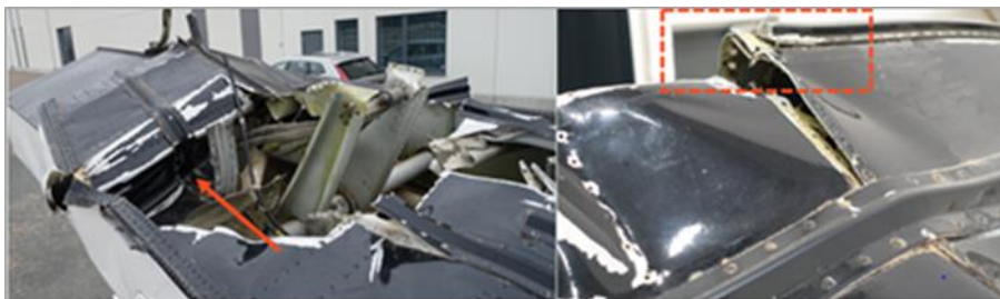
Figure 25. The left picture shows the damage to the keel. The arrow points to the pushed back keel plates. The right picture shows the bent and broken keel bar. The fuselage is upside down in the picture.
